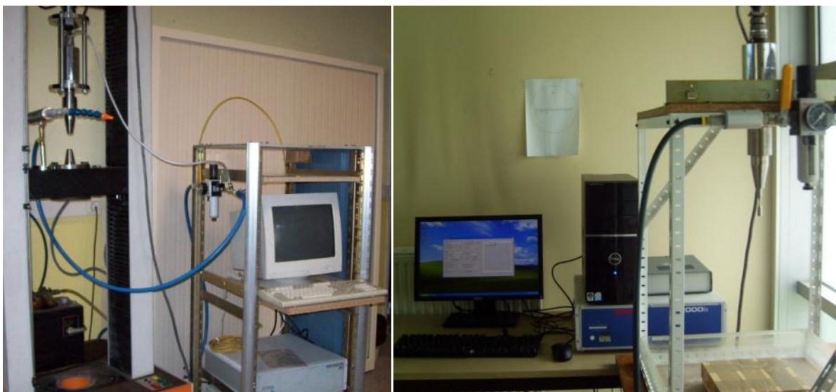
Figure 2.1. Ultrasonic fatigue testing machine at 20 kHz from Prof. Bathias laboratory (left) installed at LAMEFIP and new model at LAMEFIP (right).
