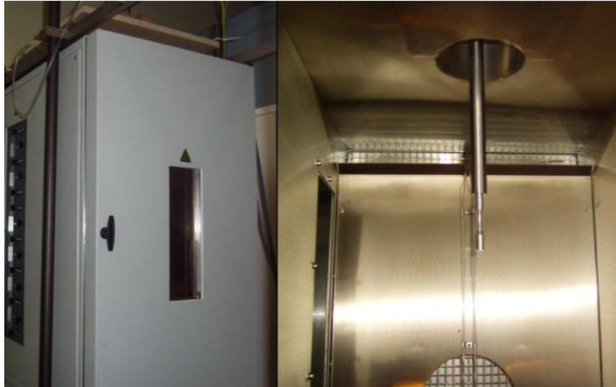
Figure 2.6. Image of the Zwick EC76B climatic chamber (right) and an internal view of a specimen in R=-1 test configuration.
