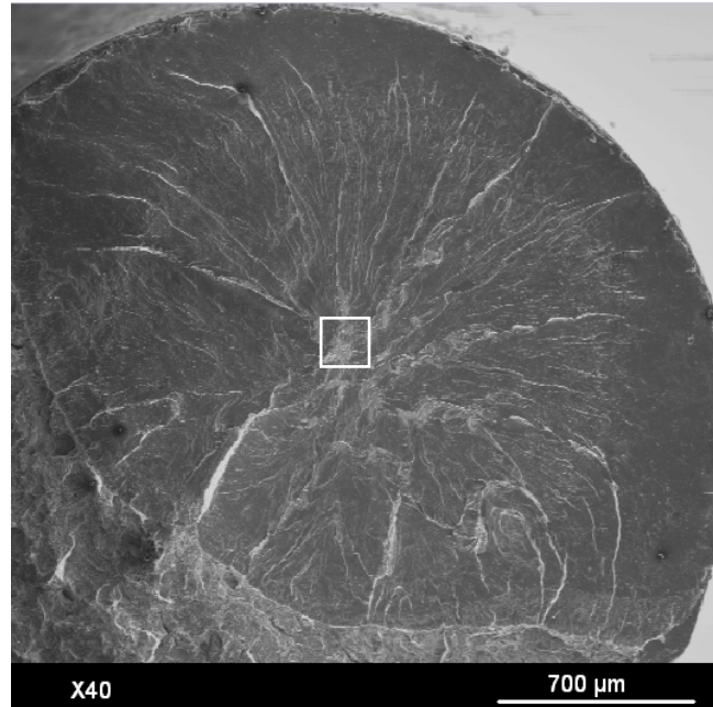
Figure 3.24. Fracture surface of a R5 steel specimen without corrosion tested at R = -1 , in air and room temperature, \sigma_a = 380\ \text{MPa} , failed at N_f = 2.78 \times 10^6 cycles.
