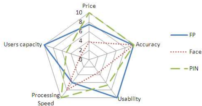
Figure 7: Comparison of fingerprint (FP), face recognition and PIN based access control systems.
