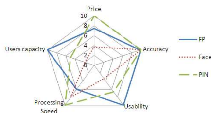
Figure 8.8: Comparison of fingerprint (FP), face recognition and PIN based access control systems.
