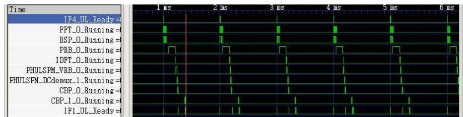
Figure 7.13: LTE uplink physical layer flow for one user
