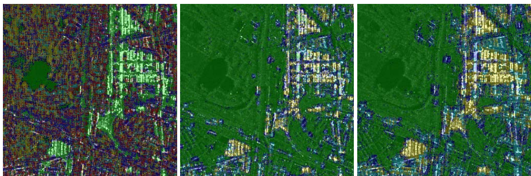
(d) Unsupervised classification based on MAP-ABM texture parameters using Model Order 4.
