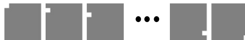
Figure 6.6: Initial space for micro patches. In each basis vector only one pixel is equal to one and other pixels are zeros
