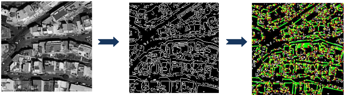
Figure 1.9: Feature extraction from a satellite image patch, using its lines properties.
