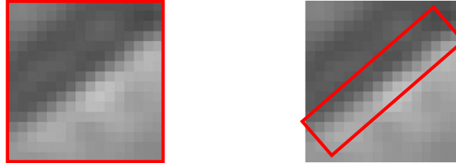
Figure 11.2: Many pixels in a square basis vector that presents a line are not necessary. We are able to represent this line by a smaller segment.
