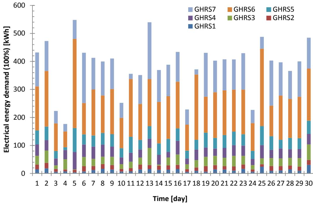
Figure 5.28 Electrical energy demand of the network of GHRS
