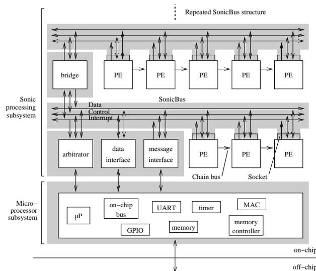
FIGURE 2.40: Architecture *Sonic-on-a-Chip*
