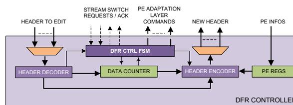
FIGURE 5.19: Architecture du *DFR Controller*
