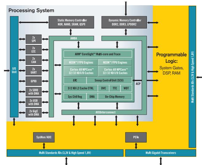
FIGURE 2.37: Architecture du ZYNQ-7000 EPP (Xilinx) [93]
