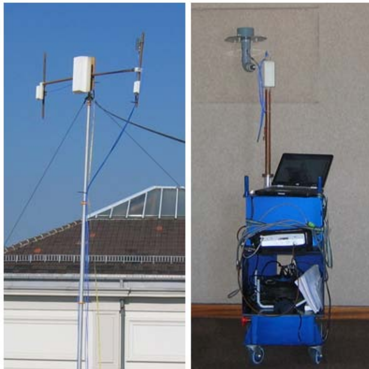
Figure 4.5: Photos of Tx antenna and Rx set-up with rotating device
