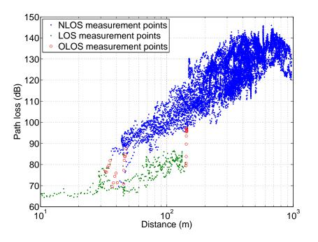
Figure A.3: LOS/OLOS/NLOS classification for RS2-MS link
