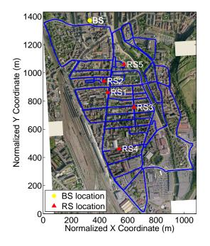
Figure 3.7: RS locations and measurement route at Train Station area
