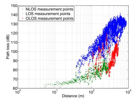
Figure A.1: LOS/OLOS/NLOS classification for RS1-MS link
