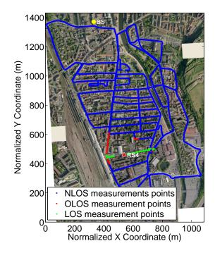
Figure A.6: RS4-MS LOS/OLOS/NLOS measurement points
