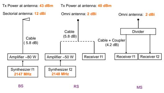
Figure 3.4: Radio configuration at BS, RS and MS
