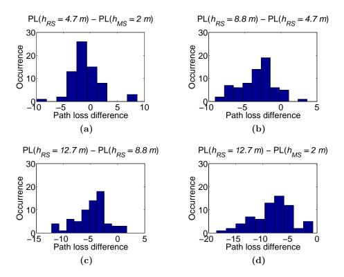
Figure 4.3: Histogram of path loss difference between RS antenna heights
