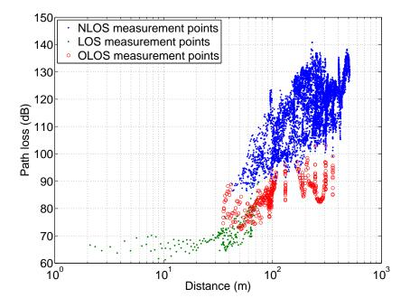
Figure A.13: LOS/OLOS/NLOS classification for RS8-MS link
