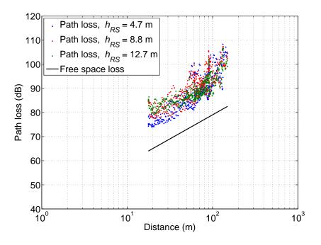
Figure C.5: RS6-MS LOS path loss with 3 RS antenna heights
