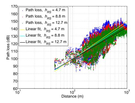
Figure B.3: RS5-MS NLOS path loss with 3 RS antenna heights
