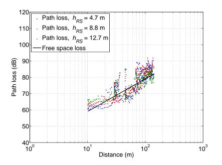
Figure C.1: RS2-MS LOS path loss with 3 RS antenna heights
