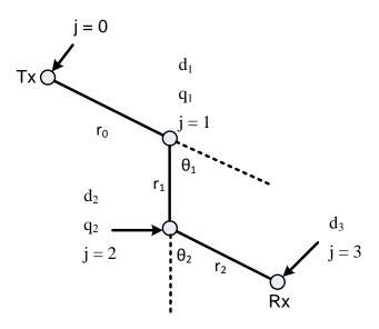
Figure 2.11: Street geometry used for Berg model
