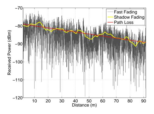
Figure 2.3: Three scales of radio mobile signal variation
