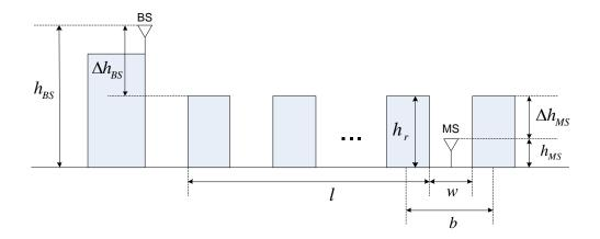
Figure 2.6: Parameters of COST-231 Walfish-Ikegami model
