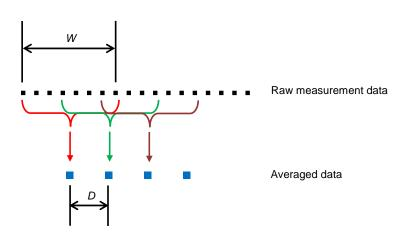
Figure 3.11: Averaging procedure of measurement signal
