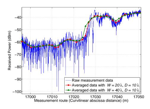
Figure 3.12: Averaged data with different W and D in comparison with raw measurement data
