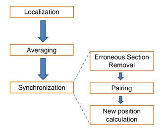
Figure 3.9: Data processing steps for BS-MS/RS-MS measurements
