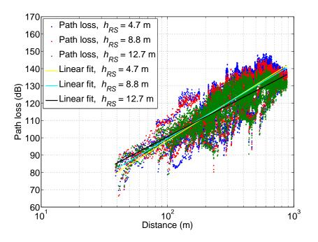
Figure 4.19: RS1-MS NLOS path loss with 3 RS antenna heights
