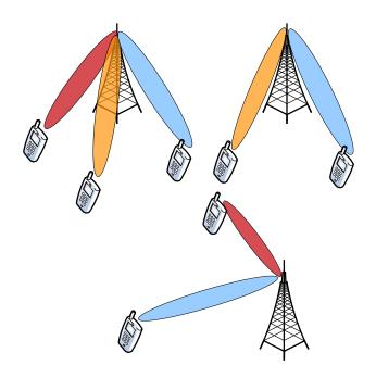
Figure 1.6: An example of CoMP with 3 collaborating cells
