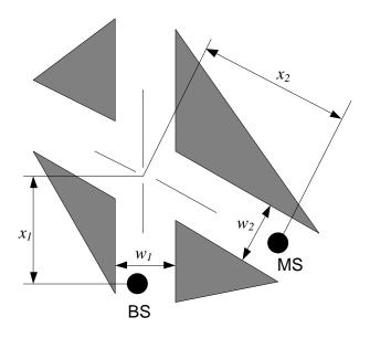
Figure 2.9: Parameter definitions for propagation within street canyons
