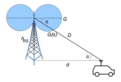
Figure 4.21: Antenna radiation pattern effects on path loss
