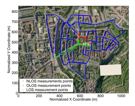
Figure A.18: RS10-MS LOS/OLOS/NLOS measurement points
