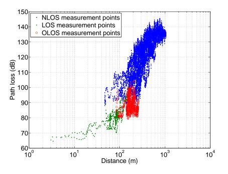
Figure A.7: LOS/OLOS/NLOS classification for RS5-MS link
