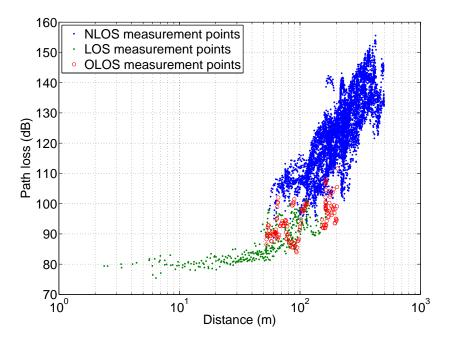
Figure A.15: LOS/OLOS/NLOS classification for RS9-MS link
