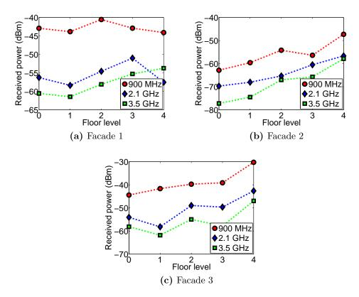
Figure 4.9: Received power dependence on floor level
