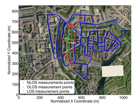
Figure A.12: RS7-MS LOS/OLOS/NLOS measurement points
