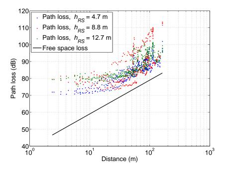
Figure C.7: RS9-MS LOS path loss with 3 RS antenna heights
