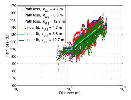
Figure B.6: RS9-MS NLOS path loss with 3 RS antenna heights
