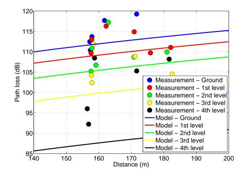
Figure 4.12: Proposed path loss model prediction in comparison with the measurements at facade 2 in the additional measurement campaign
