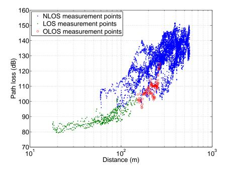
Figure A.9: LOS/OLOS/NLOS classification for RS6-MS link
