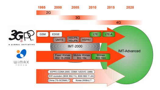
Figure 1.1: Evolution of radio mobile systems
