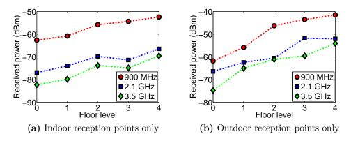
Figure 4.7: Received power dependence on floor level
