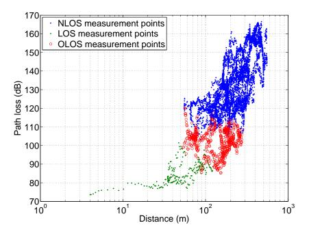
Figure A.11: LOS/OLOS/NLOS classification for RS7-MS link
