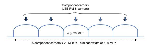
Figure 1.4: A continuous carrier aggregation example
