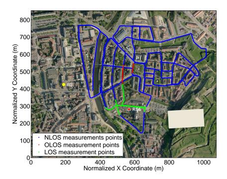
Figure A.10: RS6-MS LOS/OLOS/NLOS measurement points
