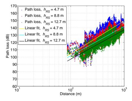
Figure B.2: RS4-MS NLOS path loss with 3 RS antenna heights
