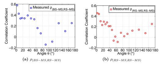
Figure 4.28: Measured SF correlation vs. angle  $\theta$
