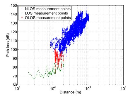
Figure A.5: LOS/OLOS/NLOS classification for RS4-MS link
