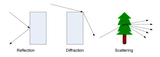
Figure 2.1: Basic propagation mechanisms
