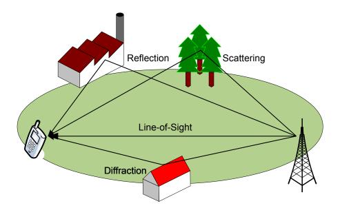
Figure 2.2: Multipath propagation
