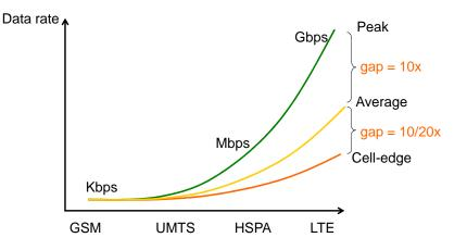
Figure 1.2: Cell-edge problem in radio mobile systems
