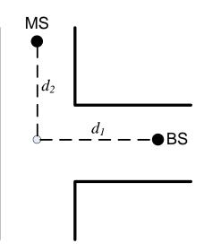
Figure 2.10: Definition of  $d_1$  and  $d_2$  for B1 path loss model
