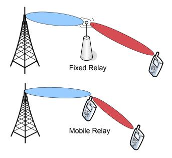
Figure 1.7: Fixed Relay vs Mobile Relay
