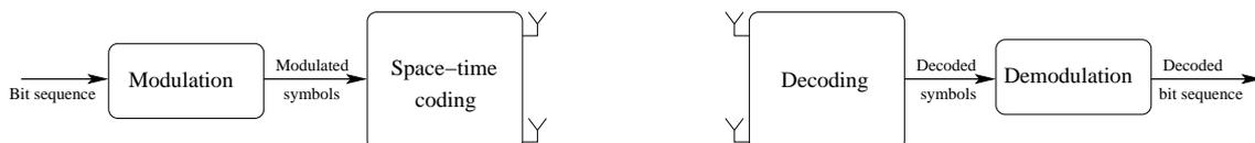
Figure 1.5: Transmission chain of a MIMO system
