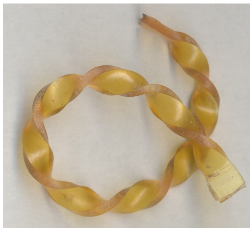
Figure 15 – The equilibrated torsade is bent into a loop at 100 °C and cooled down below T_g . If we heat it up above T_g again, it will retrieve its straight twisted shape.
