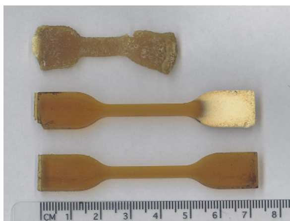
Figure 13 - Photos of injection-molded N-5% samples from top to bottom: a) injection in cold mould for 30 s (25°C), b) injection in mould heated at 200°C for 30 s and left to cool down to 25°C for 6h. NB: the whitish left part of the sample is only an issue at the surface and cohesion is maintained in the bulk of the sample. c) injection in mould heated at 200°C for 30 s and water-cooled down to 25°C in 5 min.
