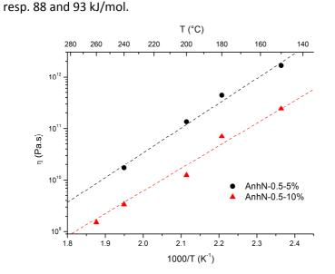
Figure 13 - Arrhenius plot of viscosities measured for samples AnhN-0.5-5% and AnhN-0.5-10% at different temperatures.
