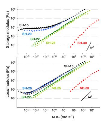
Figure 4 – Time-temperature superposition of rheological mastercurves: Storage (top) and Loss (bottom) modulus obtained from small deformations oscillatory experiments.
