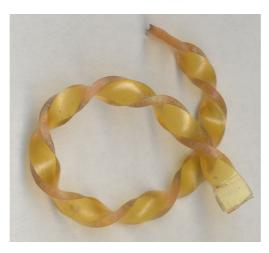
Figure 15 – The equilibrated torsade is bent into a loop at 100 °C and cooled down below Tg. If we heat it up above Tg again, it will retrieve its straight twisted shape.
