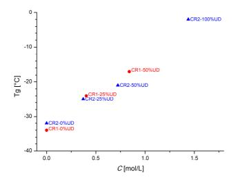
Figure 10 - Tg of the different crosslinked samples as measured by DSC.
