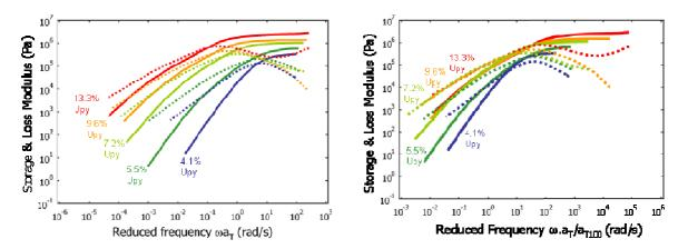
Figure 17 - Rheological master curves of PBA modified with Upy. Data was taken from Ref. 18. Storage and loss modulus are shown resp. in plain and dotted lines. (left) mastercurves are referenced at 50°C. (right) mastercurves are referenced at Tg + 100°C.
