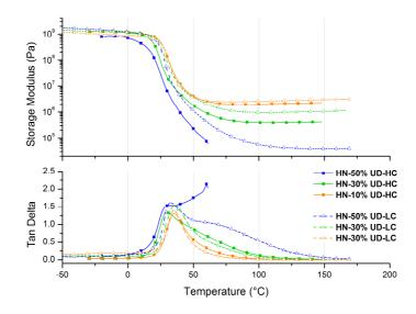
Figure 6 - DMA traces (1Hz) of Storage modulus and tan δ versus temperature for HN-10%UD, HN-30%UD and HN-50%UD. Solid lines: samples with low catalyst concentration, dotted lines: samples with high catalyst concentration.
