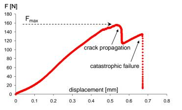
Figure 7 – Schematic representation of a shear-lap experiment with a high Tg material.
