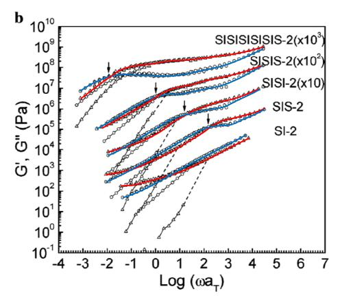
Figure 18 - Master Curves of multiblock Styrene-Isoprene copolymers taken from Ref 33. Red and Blue lines mark the storage and loss modulus obtained for T <  $T_{ODT}$ . Non-marked data were taken at T >  $T_{ODT}$ , i.e. when no long-range ordering can be seen. Triangles and Circles resp. are used for G' and G". Note that the master curves for SISISISISIS-2 (top), SISIS-2, and SISI-2 are respectively vertically shifted by factors  $10^3$ ,  $10^2$  and 10.
