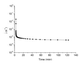
Figure 12 - Evolution of the strain rate with time for the sample AnhN-0.5-10%, at 200 °C. Strain-rate attains a constant value of  $\dot{\gamma}$  = 4.03×10<sup>-5</sup> s<sup>-1</sup>, the viscosity calculated is η=1.2×10<sup>10</sup> Pa.s.
