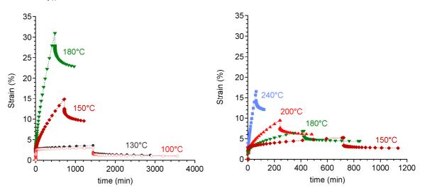
Figure 11 – Creep experiments for 0.5 MPa, at different temperatures, conducted on samples AnhN-0.5-5% (left) and AnhN-0.5-10% (right)
