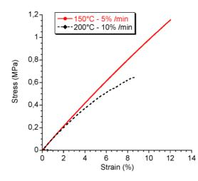
Figure 10 - Stress-strain curves of sample AnhN-0.5-10%. Strain rates of respectively 5%/min and 10%/min are applied at 150 and 200°C. Elongation at break is about 10%.
