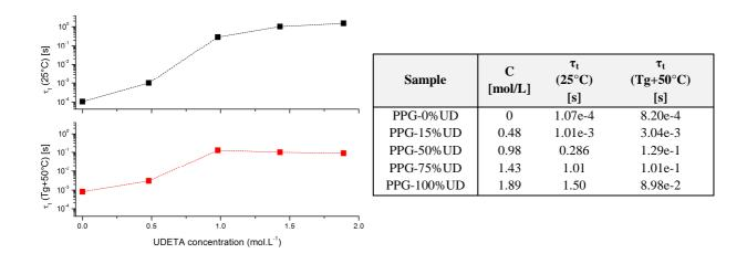
Figure 15 - Terminal times ( $\tau_t=2\pi/\omega_t$ ) measured for different concentrations of UDETA, from TTS curves referenced at 25°C (top) and at Tg+50°C (bottom).
