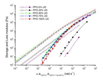
Figure 14 – Time-temperature superposition curves referenced at Tg+50°C for samples PPG-0%UD, PPG-25%UD, PPG-50%UD, PPG-75%UD, PPG-100%UD. Storage and loss modulus are shown in filled and open symbols.
