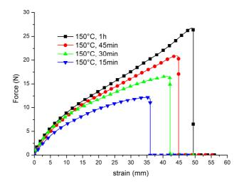
Figure 9 - Tensile tests carried out on assemblies from epoxy-acid networks catalyzed with Zn(Ac)2 at 5 mol%, and mended at 150 °C for different times.
