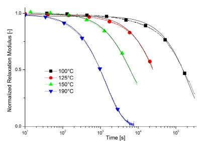
Figure 5 – Normalized stress-relaxation data (G(t)/G0) for epoxy-acid networks, catalyzed with Zn(Ac)2 (5 mol%). The data was fitted at different temperatures with mono-exponential models (in black).
