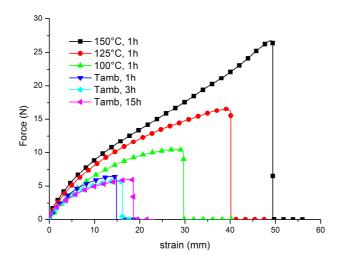
Figure 8 - Tensile tests carried out on assemblies from epoxy-acid networks catalyzed with Zn(Ac)2 at 5 mol%, and mended for 1 h at different temperatures.
