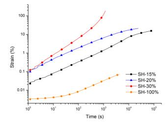
Figure 5 - Creep measurements for samples SH, conducted at 30 °C with a 3 kPa stress.
