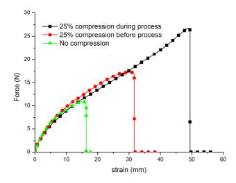
Figure 11 - Tensile tests carried out on assemblies from epoxy-acid networks catalyzed with Zn(Ac)2 at 5 mol%, mended for 1 h at 150 °C. triangles: no pressure was applied to maintain the assembly; circles: a 25% compression was applied 2 hr at 25 °C and released before mending ; squares: a 25 % compression was applied during the mending process.
