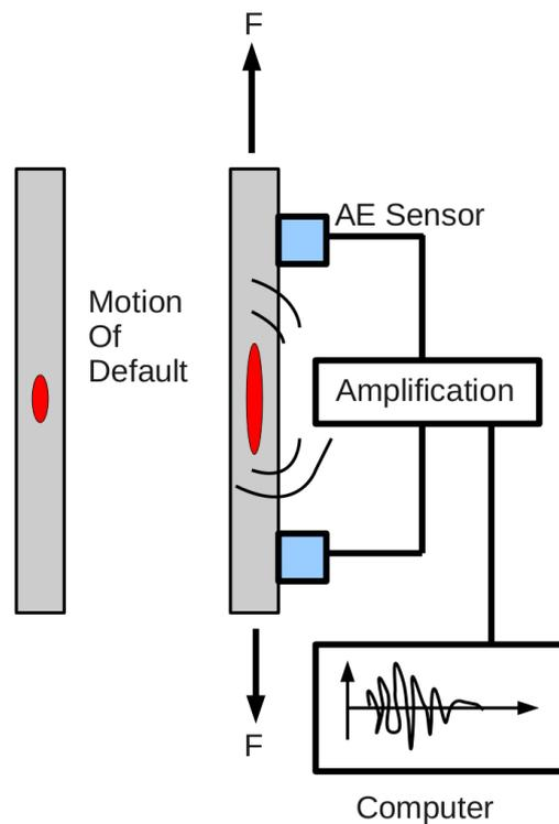
Figure A.1 – Scheme of acoustic measurement devices
