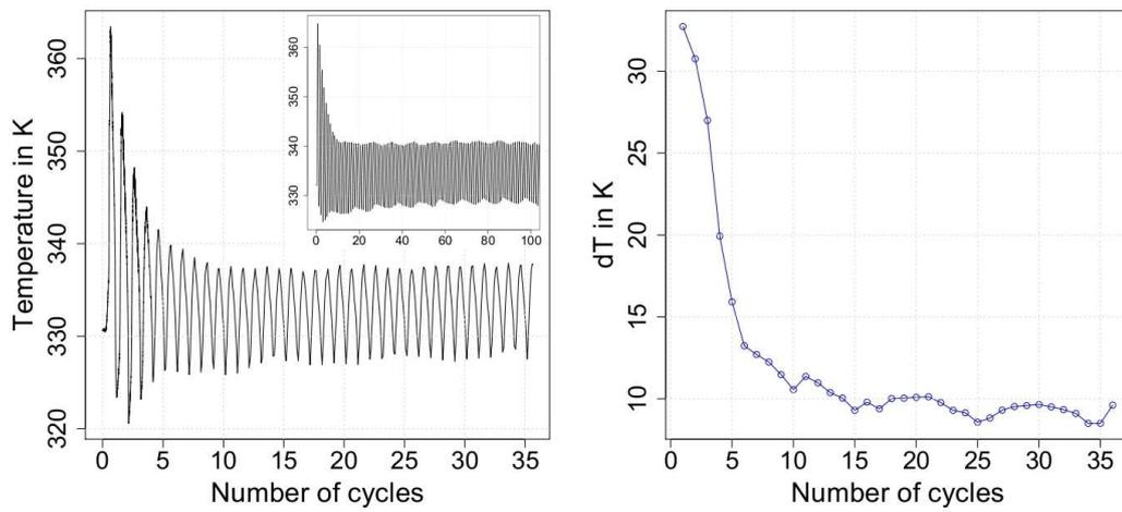
Figure 3.3 – Evolution of the variation of temperature for a given location in the sample (left) and amplitude of the variations of temperature per cycle (right)
