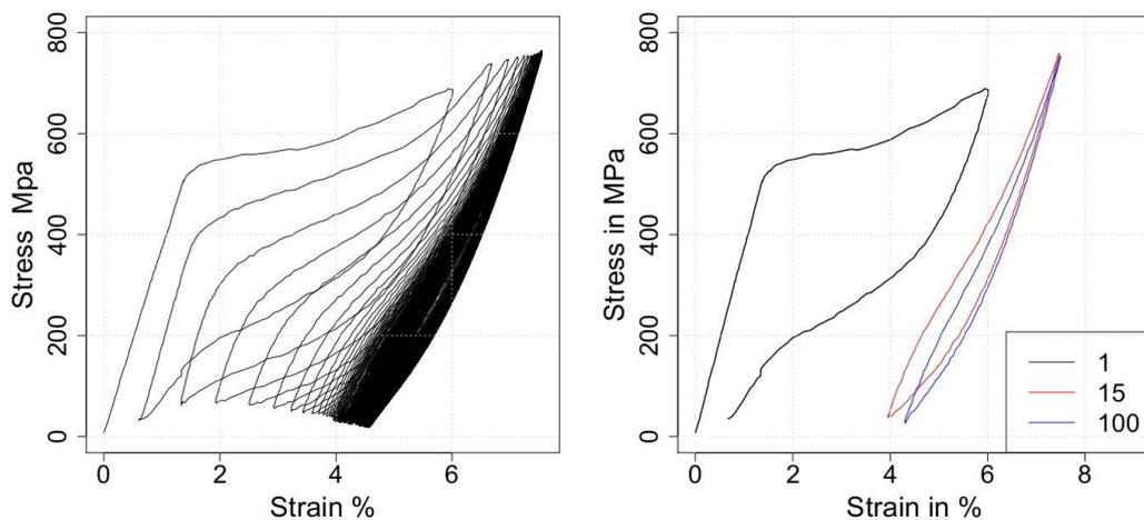
Figure 3.1 – Cyclic stress strain curves
