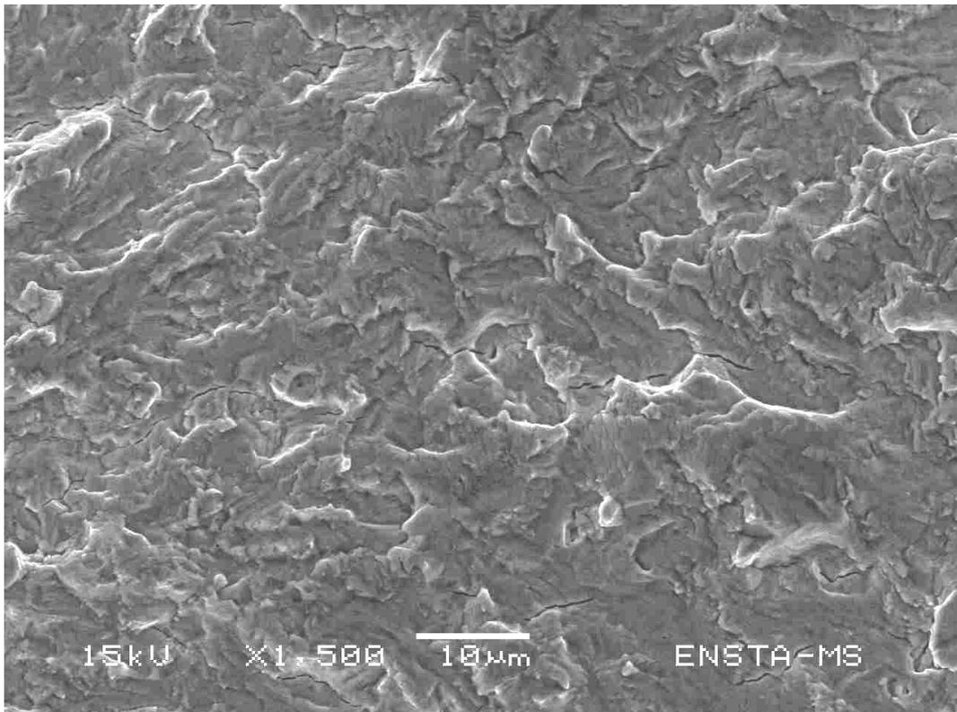
Figure 4.35 – Visualization of the secondary micro-cracks (Area B)
