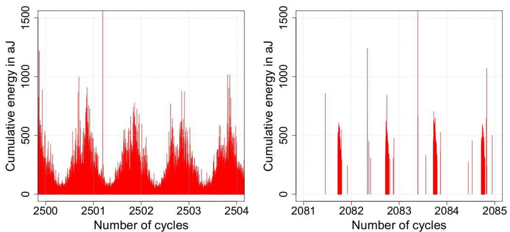
Figure 4.24 – Acoustic patterns of the development of cracks for the 4<sup>th</sup> and 9<sup>th</sup> experiment
