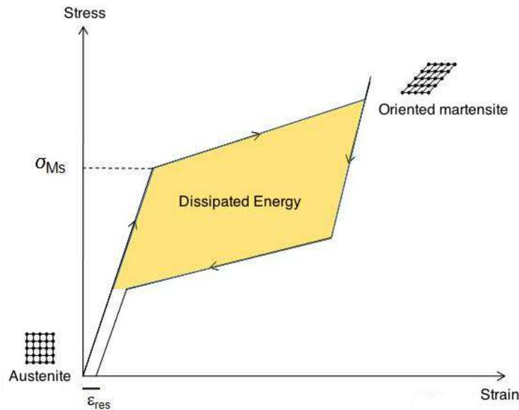
Figure 2.3 – Three main variables of hysteresis loop
