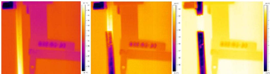
Figure 4.30 – Infra-red photos taken at (-20)ms, at 0 ms and (+20)ms from the breaking of the sample
