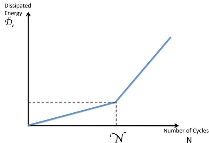
Figure 4.37 – Theoretical response of the acoustic dissipated energy of a repeatedly loaded SMA
