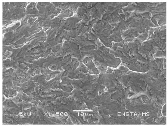
Figure 4.35 – Visualization of the secondary micro-craks (Area B)
