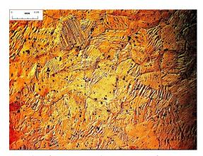
Figure 3.14 – Micrography of a NiTi sample at a strain of 0.7%
