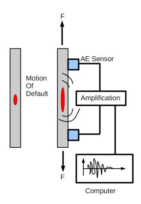
Figure A.1 – Scheme of acoustic measurement devices
