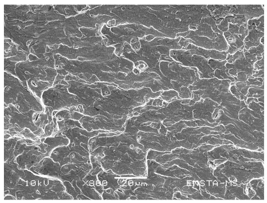
Figure 4.33 – Visualization of the area B, micro-cracks and fatigue stria
