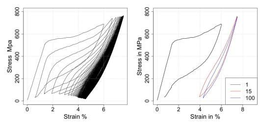
Figure 3.1 – Cyclic stress strain curves
