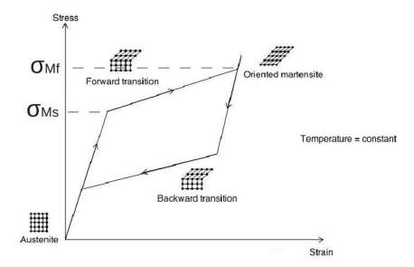
Figure 2.2 – Schematic representation of a pseudo-elastic loading
