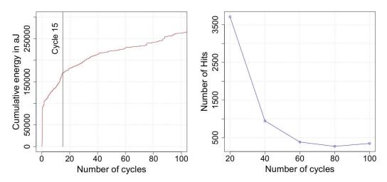
Figure 3.7 – Acoustic cumulative energy as a function of time and number of acoustic waves
