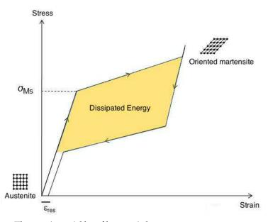
Figure 2.3 – Three main variables of hysteresis loop
