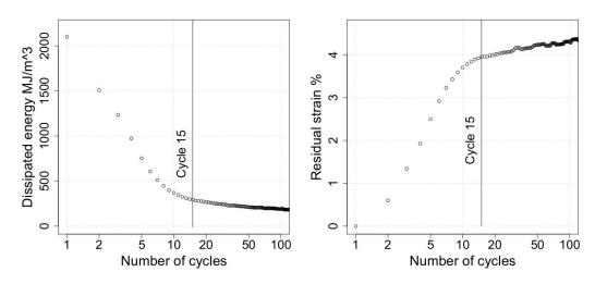
Figure 3.2 – *Dissipated energy (right) and cumulative residual strain (left) as a function of the number of cycles*
