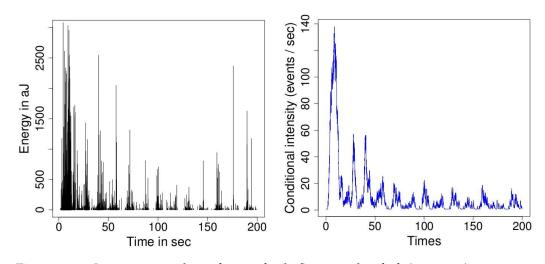
Figure 5.13 – Instantaneous release of energy for the first 10 cycles of a fatigue experiment and fitted conditional intensity
