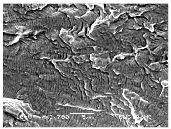
Figure 4.34 – Visualization of the fatigue stria (Area B)
