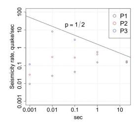
Figure 4.27 – Seismicity rate in P1, P2 and P3 - Omori's law
