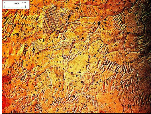
Figure 3.14 – Micrography of a NiTi sample at a strain of 0.7%
