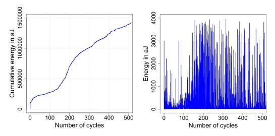
Figure 4.3 – *Cumulative energy (left) and instantaneous release of energy (right) between cycles 1 and 500*
