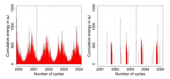
Figure 4.24 – Acoustic patterns of the development of cracks for the  $4^{th}$  and  $9^{th}$  experiment
