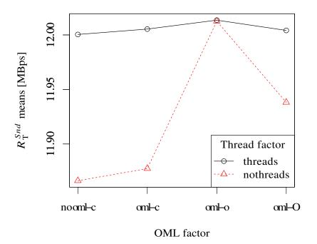
**Figure 5.5** Graph of means for the interaction between experimental factors on  $R_t^{Snd}$  at 95 Mbps. Legacy OML reporting allows unthreaded Iperf to achieve a throughput with no significant difference from the threaded version (see Table 5.5).
