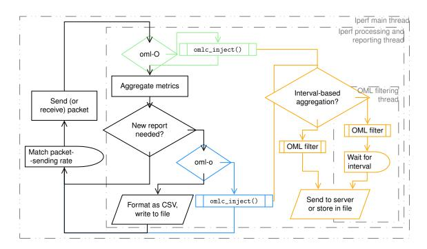
**Figure 5.3** Iperf main loop (black) and OML instrumentation additions (colours). OML reporting is implemented in two sections. The legacy mode (oml-o, blue) reports aggregate metrics computed by Iperf, while the advanced mode (oml-O, green) reports each packet. In both cases, the data can be filtered before being sent for storage (orange). Iperf can delegate reporting to a second thread if activated, while OML uses a filtering thread for time-based aggregates (*e.g.*, per-second averages).
