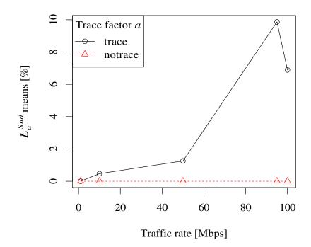
Figure 5.8 Graph of means for the interaction of factors trace and rate on the loss ratio  $L_a^{Snd}$ .
