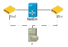
Figure 5.4 Experiment topology. An Iperf sender Snd generates traffic towards a receiver Rcv on a link capacity-shaped using NetEm. When OML applications are used, measurements are sent over the control network to OML server o.
