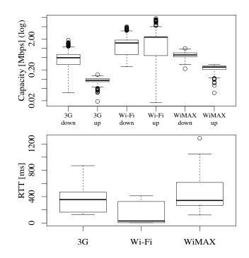
Figure 3.8 Empirical QoS distributions as measured from the testbed. Top: upstream and downstream capacity, bottom: RTT. Boxes show the 25–75% inter-quartile range (IQR), the heavier line represents the median of the data-set and whiskers extends to the extreme data within 1.5IQR from the median. Circles denote outliers.
