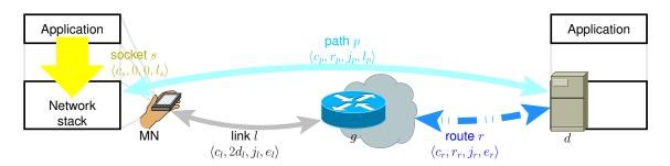
Figure 3.5 Three main elements contribute to the performance of network path p from the perspective of an application running on an MN: the first hop on the local link l, the route r from the operator network to the destination, and the socket interface between the application and the network stack s. Capacity, delays (RTT and jitter) and loss metrics are represented as a tuple for each element.
