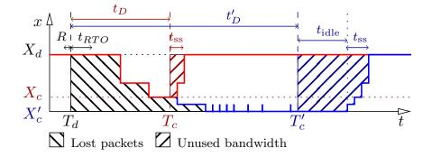
Figure 4.7 TFRC rate behaviour in a period with no connectivity. Two cases are shown, with different times of reconnection: at  $T_c$ , a time  $t_D$  has elapsed which is short enough that TFRC's rate didn't reach its minimum (red) and at  $T'_c$ , when the time  $t'_D$  elapsed since the disconnection was sufficient for X to reduce to  $s/t_{\rm mbi}$ , an additional delay  $t_{\rm idle}$  is present in this case before TFRC starts restoring its rate (blue).
