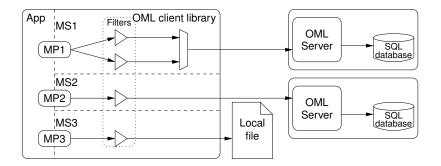
Figure 5.2 Measurement data path in OML: Three measurement streams (MS) are filtered to generate measurement streams (MS) which get stored at different locations.
