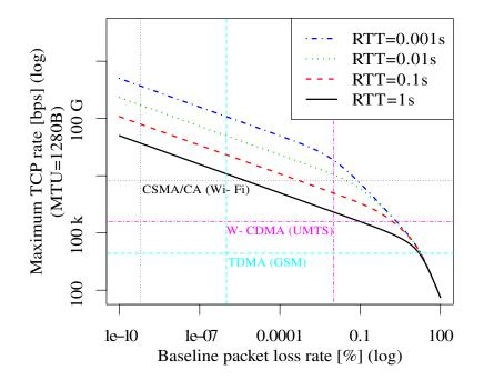
Figure 3.6 TCP's maximum throughput under various delay and loss conditions. Typical capacities and loss rates (after retransmissions) for TDMA (GSM) and CDMA/CA (Xylomenos *et al.*, 2001), and W-CDMA (UMTS; Prokkola *et al.*, 2009) are reported. They suggest that these errors alone may be ignored as a throughput-limiting factor for TCP.
