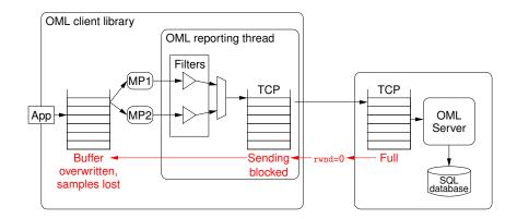
Figure 5.9 Data path from injection to database. When the transaction takes place on the server side, the TCP receiver buffer fills up. As a result a null **rwnd** is advertised to the client, which results at the other end in data discarding in the application.
