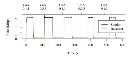
Figure 4.5 DCCP/TFRC data stream moving through non-adjacent Wi-Fi access networks.
