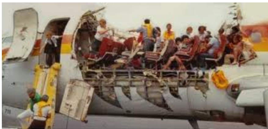
Figure 1.1: Example of corrosion occurred in 1988 on an aircraft flying between the Hawaiian islands. This disaster prompted the aircraft industry to investigate SCC phenomenon involved near sea environments ( http://www.securiteaerienne.com ).
