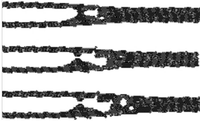
Figure 1.6: Three states of crack growth by molecular dynamics (Vamvakopoulos and Tanguy 2009)
