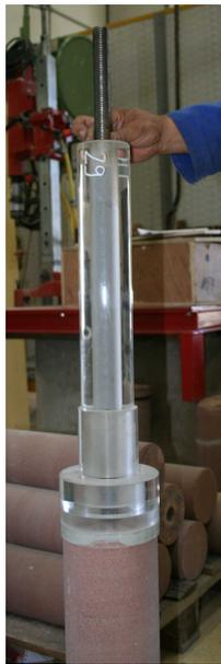
(a) test sample during the setting time of the grouting material (with centring pattern installed).
