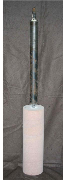
**Figure 3.12:** laboratory sample ready for a pull-out test.
