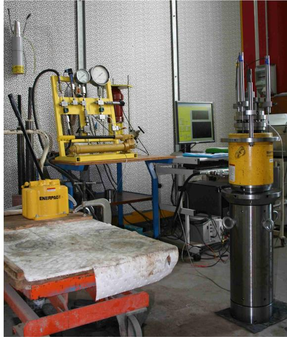
**Figure 3.2:** view of the experimental installation during a pull-out test.
