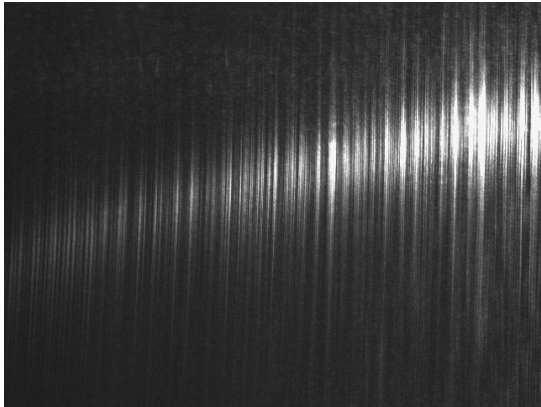
Fig. III.18. Left half of the m-line of a TIPE:LiNbO 3 waveguide with a 45° outcoupler prism. The outcoupled beam itself is situated on the right of the figure.
