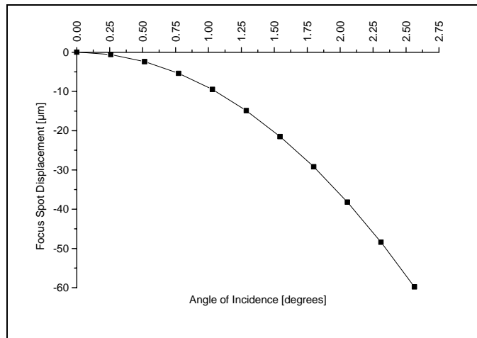
Fig. III.14. Transverse image line inclination of Lens 3.1.
