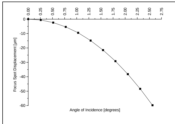
Fig. III.14. Transverse image line inclination of Lens 3.1.
