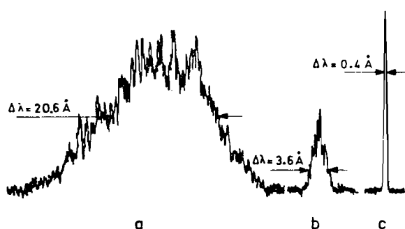
FIG. 2. Bandwidth of the laser emission. (a) Without birefringent filter in the laser cavity; (b) with one calcite plate of thickness 1 mm; (c) with two calcite plates of thickness 1 and 4 mm.
