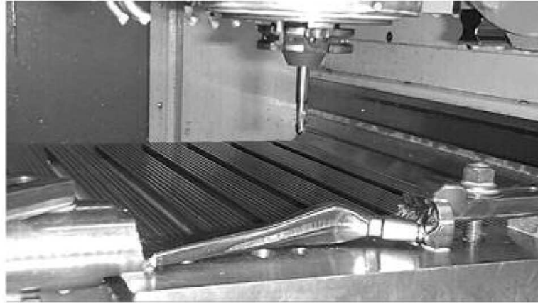
Figure 2.40: Machining of the endoprosthesis using a CNC milling (Dietrich & Skalski, 2004)
