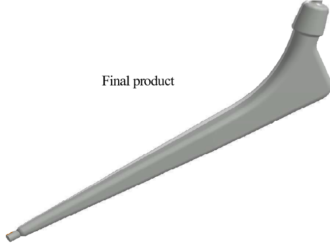
Figure 3.20: Final workpiece obtained after material removal from both sides of the workpiece
