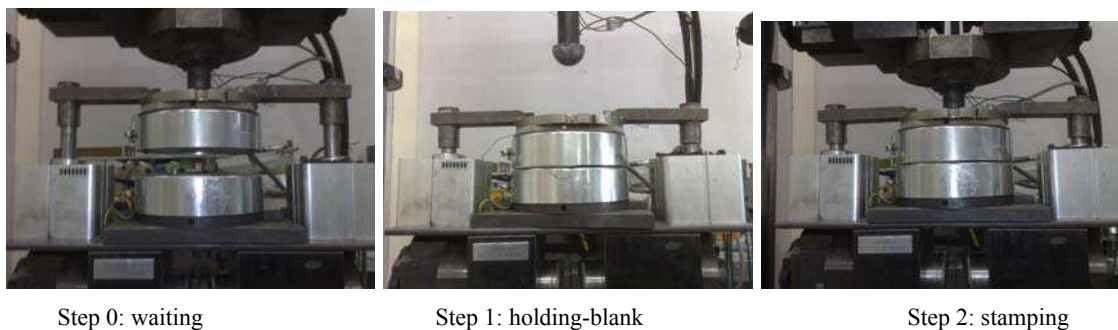
Fig.2. The procedure of the Nakazima stamping tests
