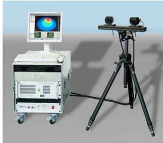
Fig.9. The ARAMIS measurement system set-up in laboratory
