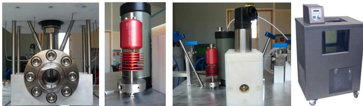
Figure 4.2. Partial pictures of the main components of the new apparatus (From left to right: Equilibrium cell, ROLSI™ sampler, pressure transducers, valve arrangement and agitation device, windowed bath).
