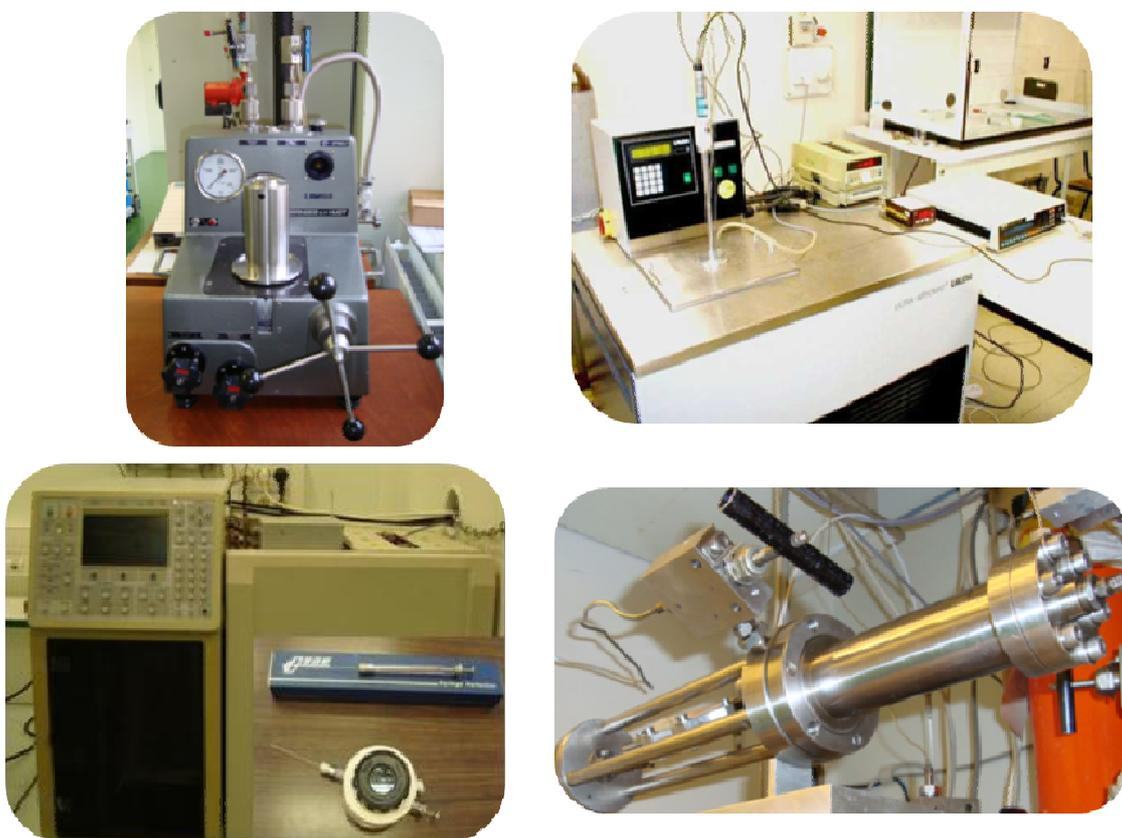
Figure 2.8. Calibration equipment used in this work: Dead weight balance device, temperature bath with reference platinum resistance thermometer probe, variable volume cell with displacement transducer for volumetric calibrations and gas chromatograph with a gas tight calibration syringe (clockwise).
