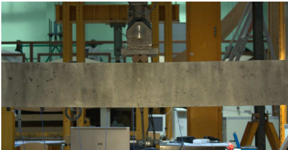
Figure 7.18: Introduction of a quasi-static load producing structural damage (cracks) at the beam's mid-span.
