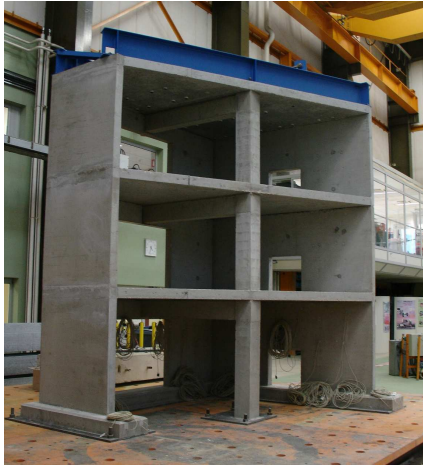
(a) Experimental specimen placed onto a shaking table at CEA laboratories
