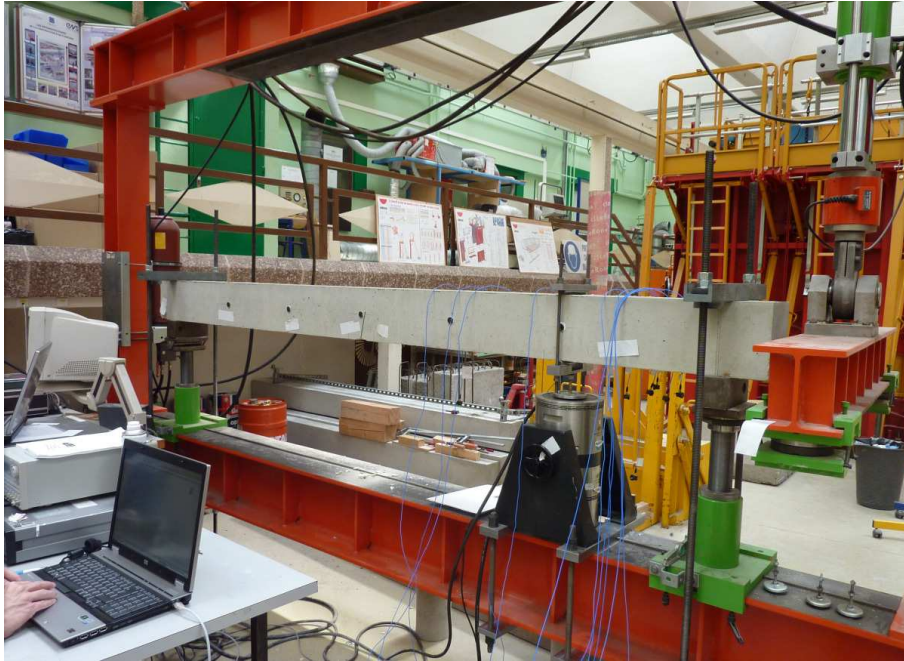
Figure 7.2: Test setup of the reinforced concrete beam with boundary coupling.
