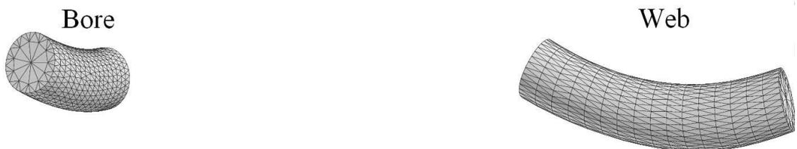
Figure V.23 : Mesh of the deformed specimens (displacement magnification factor = 100)
