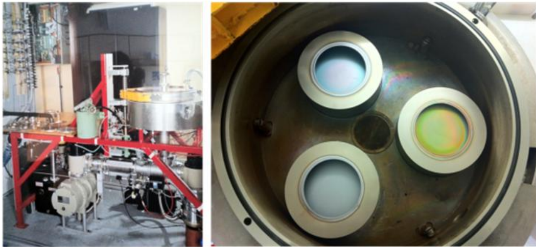
Figure 2.1 – Photo of ARCAM reactor and inside of vessel. Three plasma chambers are seen.
