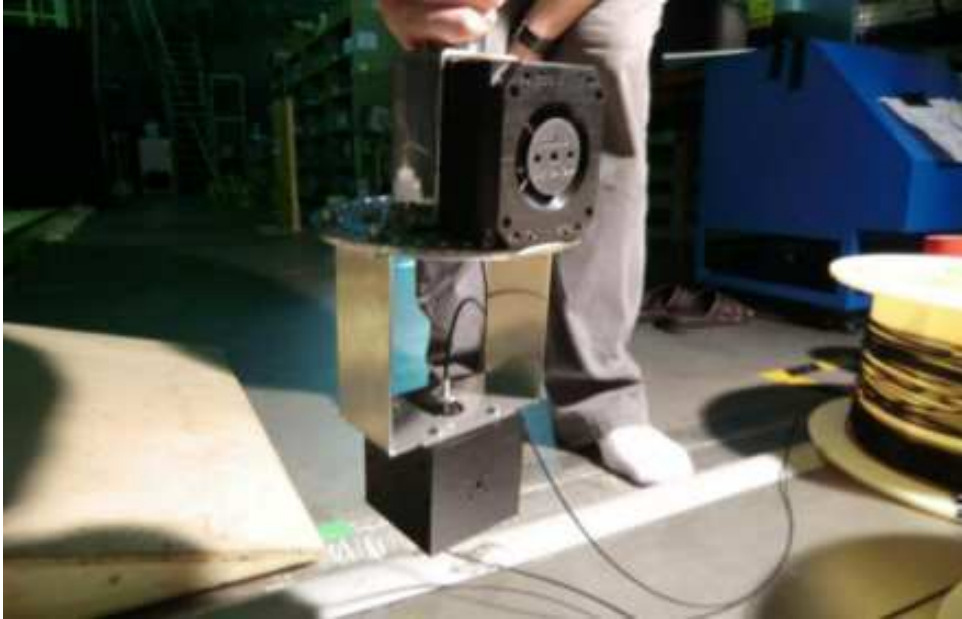
Figure 3.22: Picture of the equipment used to lower the CG vessel and Locator vessel into SK. The poles from the pole system are connected on top of the “U” shaped metal plate covering the CG vessel sides. This “U” shaped metal plate is screwed to the disk, which itself is screwed both to the CG vessel and to the lower part of the disk, lower “U” shaped metal plate, to which the Locator is screwed. This picture was taken before inserting the CG for the 2011 data taking at SK.
