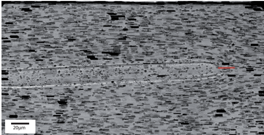
Figure D.2: Stack of frames shifted in space to be in the reference system of the fiber. The difference of velocity between the particles and the fiber makes the particles leave a path on the image stack. Black marks correspond to dust and defects in the channel.
