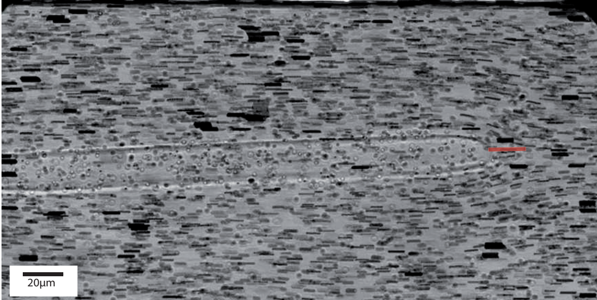
Figure 5.7: Particle paths around a fiber flowing parallel to the flow direction at a confinement of 0.4. The image is built from successive frames of the flow superimposed in the reference system of the fiber. Particles flowing above the fiber appear as still particles when others leave a trace corresponding to streamlines. We can visualize the flow around the fiber and the perturbed streamlines downstream of its edge. The perturbation extends over a distance comparable to the fiber width (and channel height).
