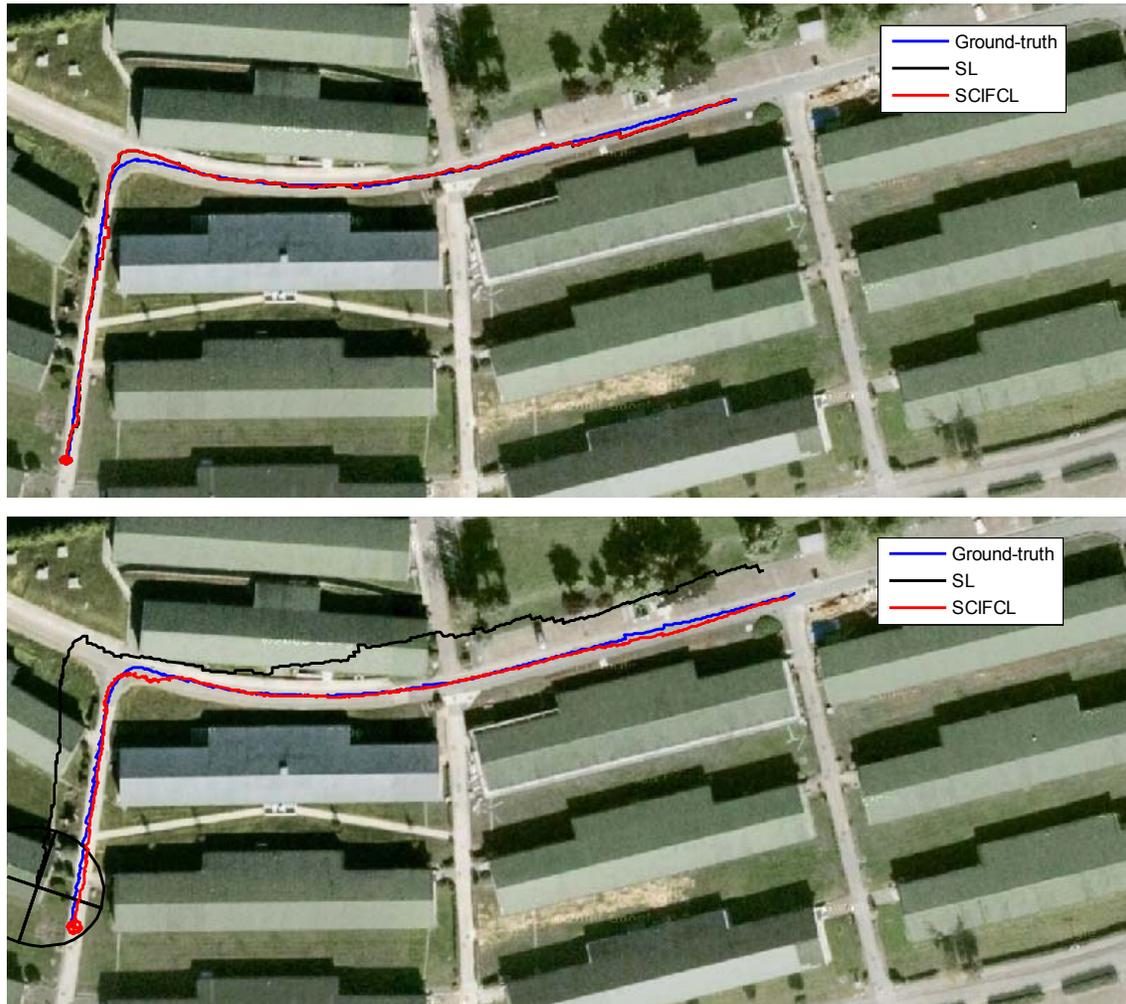
Figure 6.12 Estimated vehicle trajectories using the CL method and the SCIFCL method at the existence of GPS bias errors: (top) the first vehicle, with better absolute positioning ability; (bottom) the second vehicle, with low-accuracy absolute positioning accuracy
