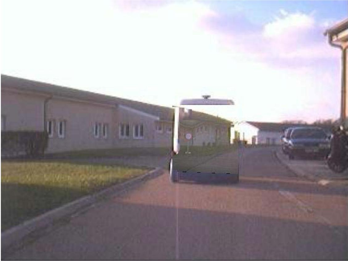
**Figure 6.34 Cooperative augmented reality effect: ‘see’ through front vehicle**
