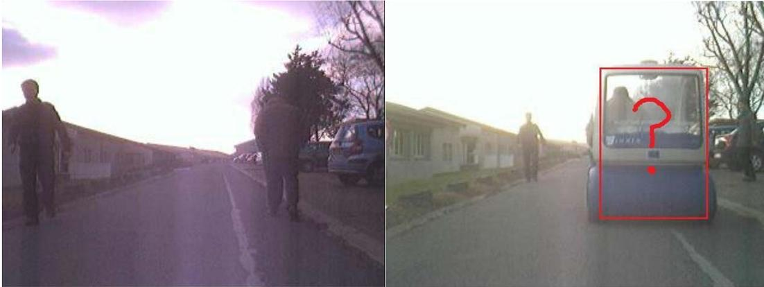
**Figure 5.1 Front-following vehicles scenario: (left) the view of the front vehicle; (right) the view of the following vehicle (occluded by the front vehicle)**
