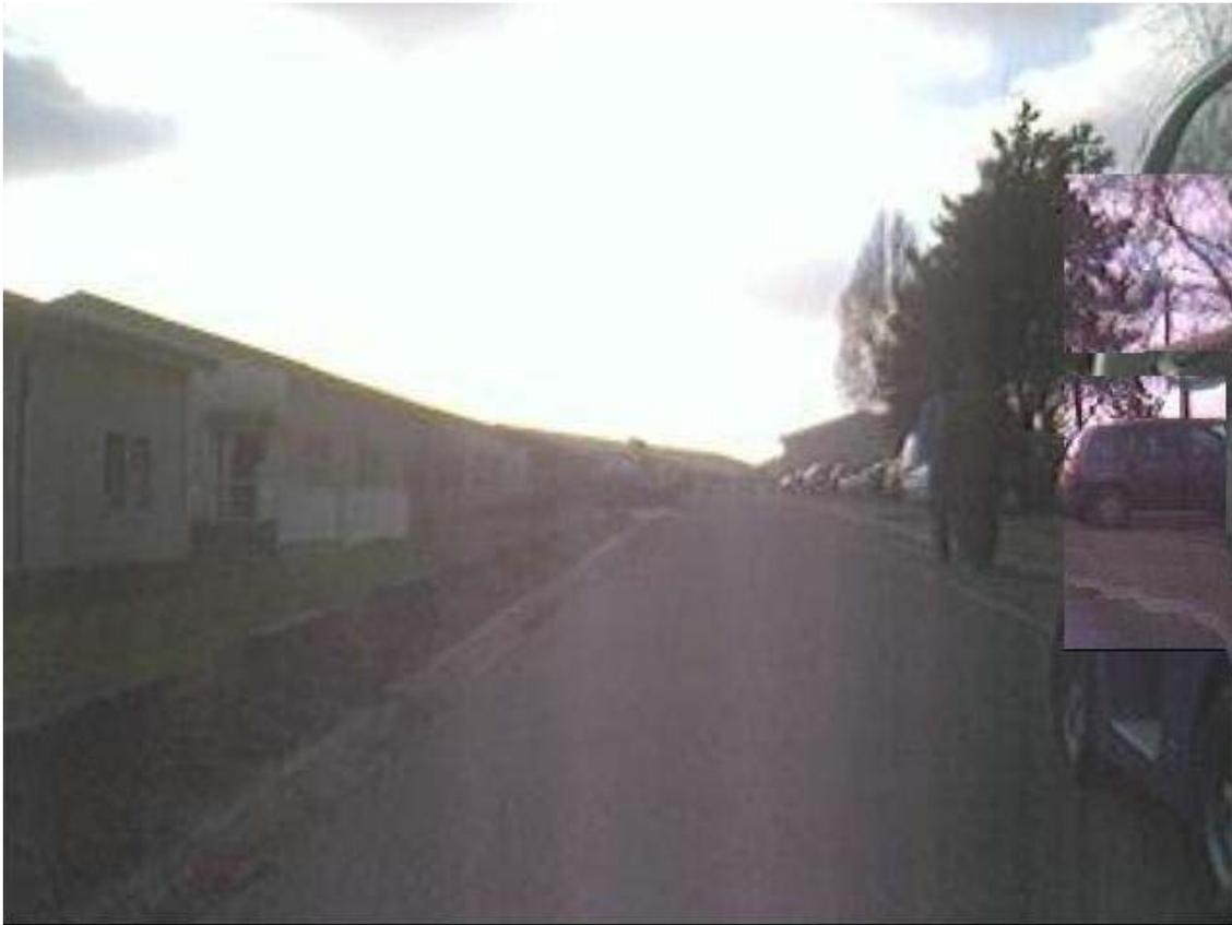
**Figure 6.31 Cooperative augmented reality effect: 'see' through front vehicle**
