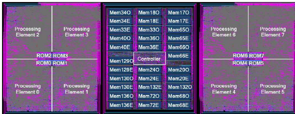
Figure 6.5. The SAR FFT floorplan[49]
