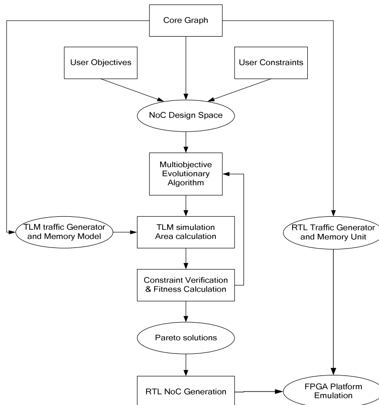
Figure 4.2. 2D NoC synthesis workflow
