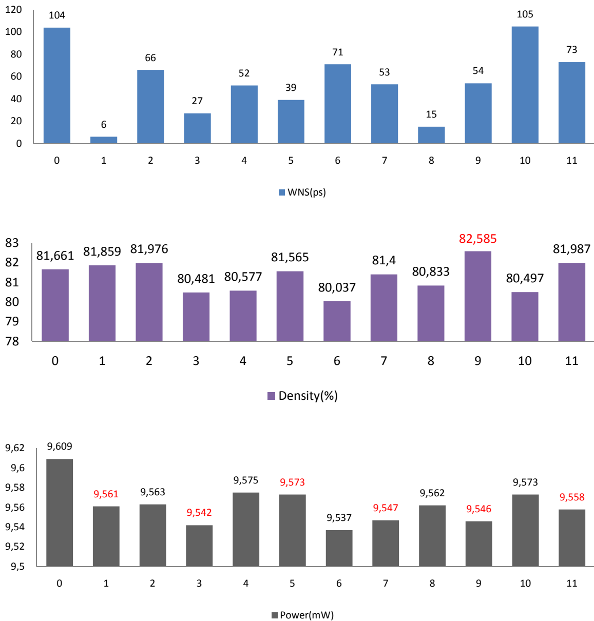
Figure 7.5.. WNS (ps), Density (%) and power (mw) for the different combinations of the DSE (Freq=100MHZ)
