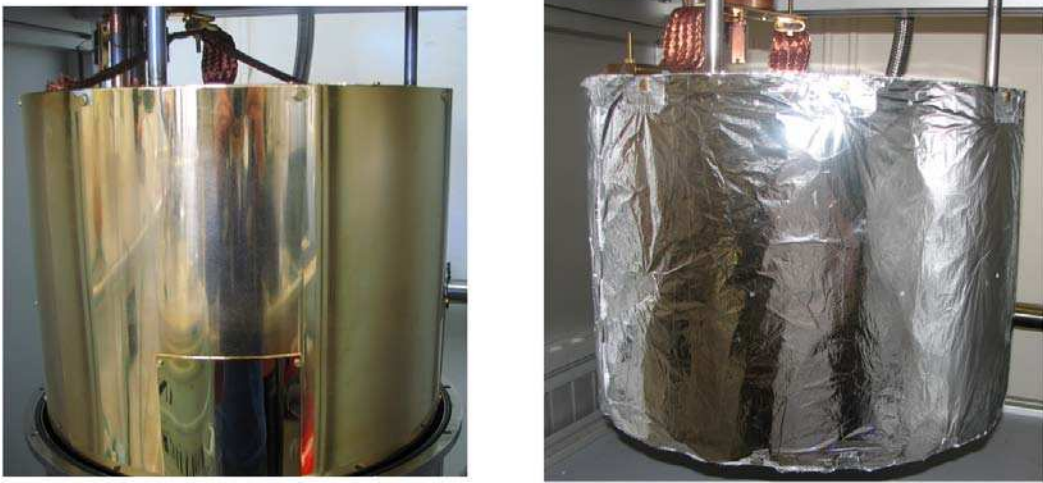
Figure 1 Multi layer insulation of the outer gold shielded copper screen with Al sheets
