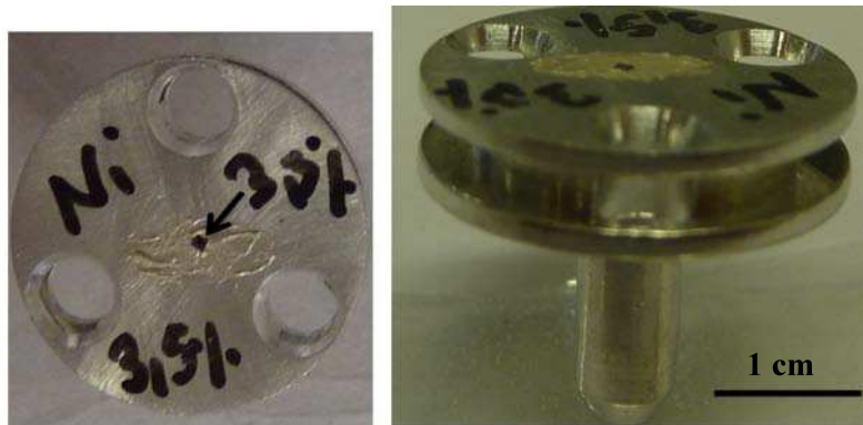
Figure 5.2 An image of crystal glued on Bitter decoration the sample holder designed in order to fit with the decoration chamber and with the SEM sample chamber. The arrow indicates the sample glued on the sample holder.
