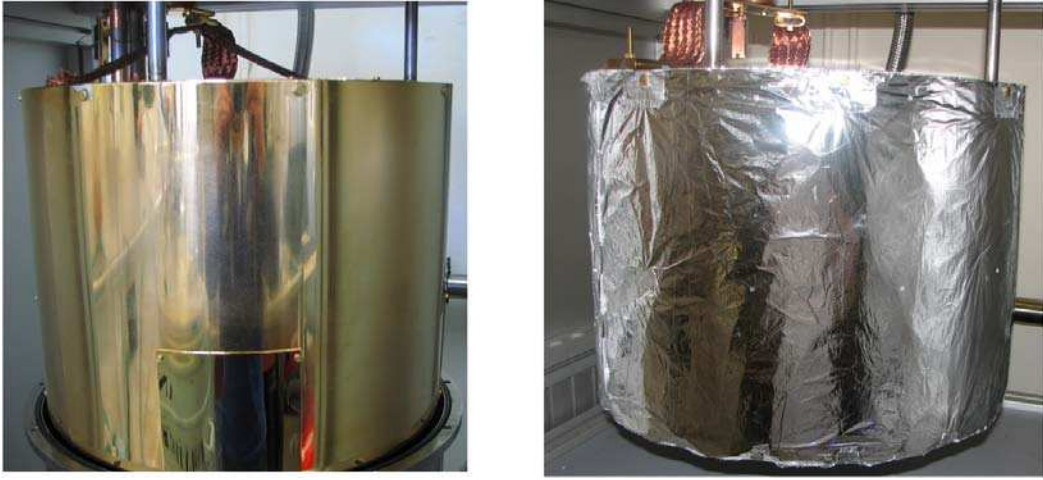
Figure 1 Multi layer insulation of the outer gold shielded copper screen with Al sheets
