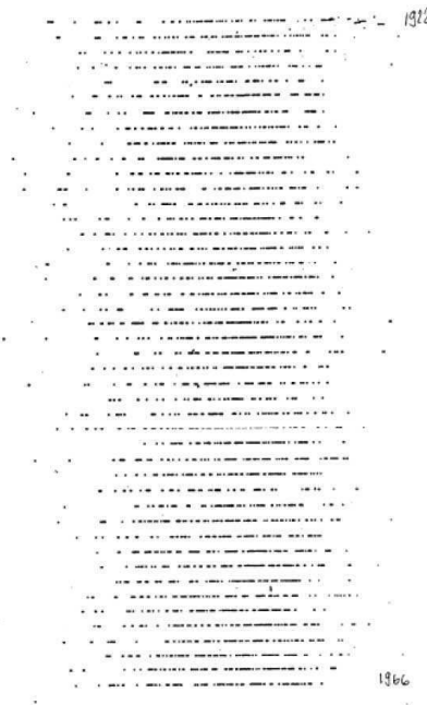
Figure 19 : Rainfall data from Dedougou for a 45 year period (1922-1966). Each line is a different year and each point a rainy day. (Hubert and Carbonnel, 1989)
