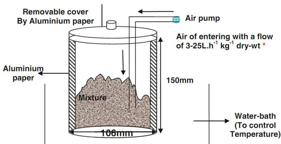
**Figure 5.1:** Design of bioreactor (volume of 1L).
