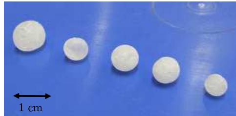
Figure 3.5: Maltodextrin spheres - Spheres of maltodextrin DE29 moulded with hands.
