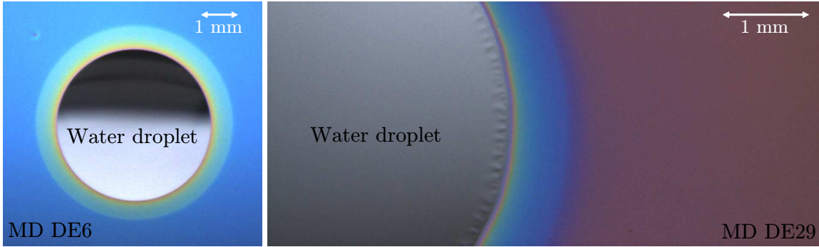
Figure 3.19: Color pictures obtained in spreading experiments - Typical pictures acquired by the color camera of spreading set-up. (left) Water droplet onto a 300 nm-thick maltodextrin DE6 layer equilibrated at a_w = 0.58 . (right) Water droplet onto a 250 nm-thick maltodextrin DE29 layer equilibrated at a_w = 0.43 .
