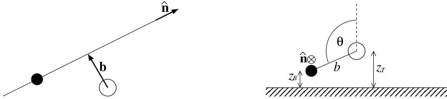
FIGURE 1. Parameters describing the scattering geometry between a swimmer (solid circle) and a tracer (open circle) in the bulk (Left) and close to a solid surface (Right). The swimmer moves in the \hat{\mathbf{n}} direction (parallel to the surface when close to it). The vector \mathbf{b} points from the initial position of the tracer to the position of minimal approach of the straight trajectory and its magnitude is b , the impact parameter. Close to a solid surface, the tracer initial height is z_T , the angle \theta gives the horizontal displacement of the swimmer trajectory with respect to the initial position of the tracer and the height of the swimmer is z_B .
