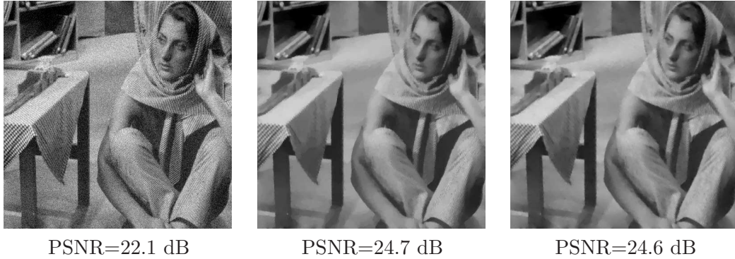
Figure 3.11: Image Barbara that underwent an addition of a white Gaussian noise of standard deviation \sigma = 20 , its TV -minimizer and its J -minimizer obtained with \lambda = 25 , respectively.
