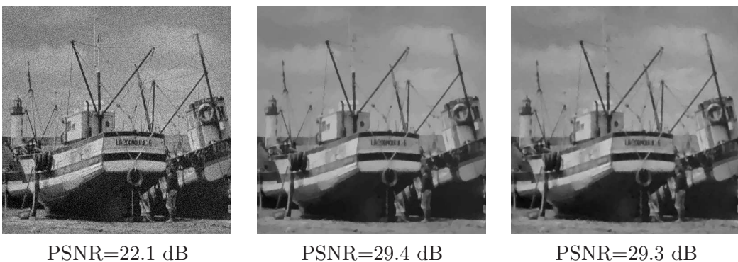
Figure 3.10: Image Boats that underwent an addition of a white Gaussian noise of standard deviation \sigma = 20 , its TV -minimizer and its J -minimizer obtained with \lambda = 25 , respectively.
