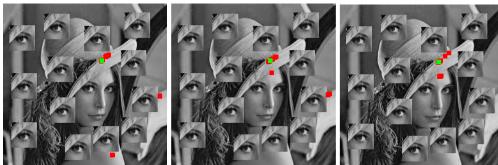
Figure 4.22: Best matches for the atom-based \delta^1 , Figure 4.23: Best matches for the ideal distance \delta^2 , Figure 4.24: Best matches for the SSD \delta^3 .
