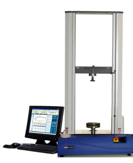
FIGURE 2.8 – Machine de force
