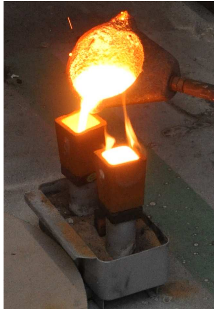
Figure 5.2: Schematic representation of standard non-tellurium cups for thermal analysis.
