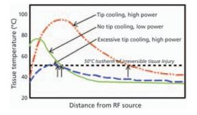
Figure 7.4: Tissue heating with regular and cooled-tip catheters. Image from [Hai08].
