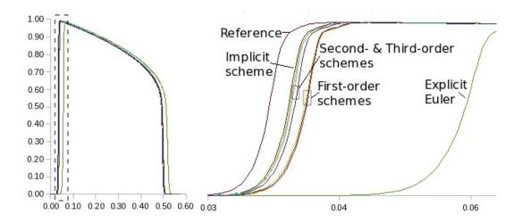
Figure B.1: Transmembrane potential u wave for MS model and zoom (dashed box), temporally integrated with different schemes, on h = 1.5mm,  $\delta t = 1ms$  in comparison with reference (abscissa: normalised potential vs time (s)).
