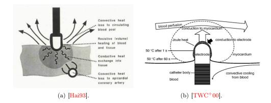
Figure 7.3: Schematics of the thermodynamic processes during RFA.
