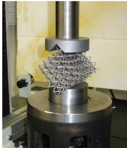
Figure C.6: Experimental setting for the compressive test of the hexatruss cell along [110]
