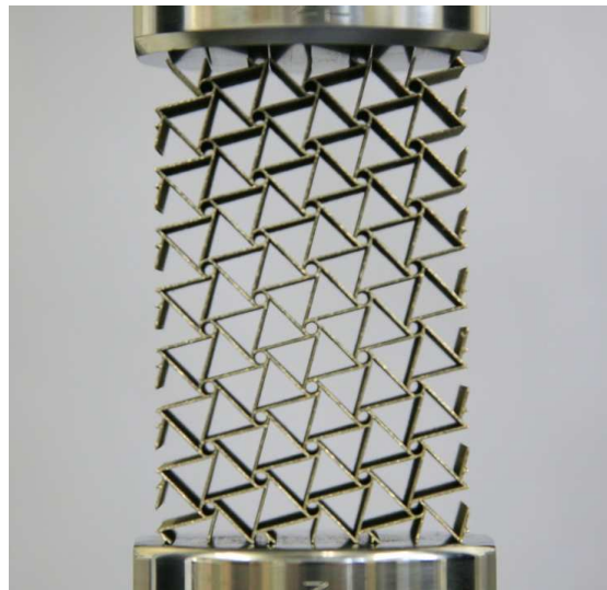
Figure C.5: Experimental setting for the compressive test of the hexachiral cell along [100]
