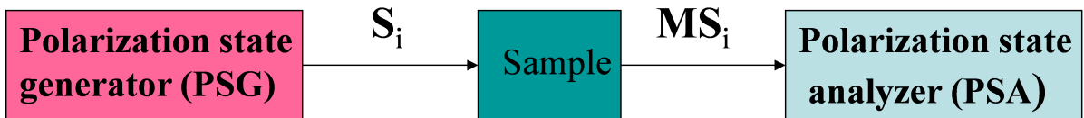
Figure 2.16: Schematic representation of the optical setup of a general Mueller ellipsometer. The Stokes formalisms has been used to represent the polarization properties of light. In the framework of Stokes formalisms the optical properties of the PSG, sample and PSA can be represented by matrices.
