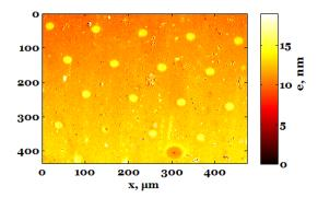
**Figure 3.17** The deposited layer thickness after the electrografting of NBD C=0.01 M in ACN +0.1 M NBu<sub>4</sub>BF<sub>4</sub> for a chronoamperometric potential step between 0.35 and -0.6 V vs Ag/AgCl for 300s, on an Au surface modified initially with 1-decanethiol (C=0.01 M) and then locally modified by UV-lithography; RIE time:2 min.
