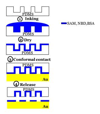
**Figure 3.2** Diagram illustrating μCP procedure for Au surface patterning with chemicals.
