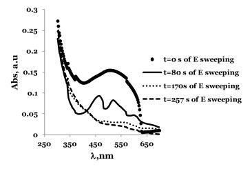
**Figure 2.17** Variation of absorption during the biasing of an electrografted ITO electrode in a solution containing only the electrolyte (0.1 M NBu4BF4 in ACN) between 0.5 et -1.2 V for 300s.
