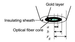
**Figure 1.13** Schematic diagram of the tip for SECM – OM coupling: a) inner radii; b) outer radii; c) outermost radii including the insulating sheath (r<sub>g</sub>)
