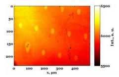
**Figure 3.5** Light reflectivity image in air of a bare Au surface modified by UV-VIS photolithography
