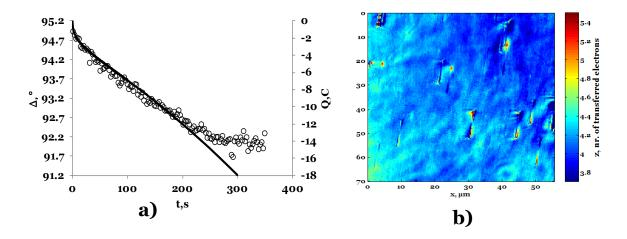
Figure 4.10 a) Variation of  $\Delta$  in degrees, averaged on a 10 $\mu$ m x 10 $\mu$ m during NBD electrograting (black open circles) correlated with consumed charge (black dashed line), for a chronoamperometric potential step between 0.2 and -0.6 V vs Ag/ AgCl for 300 s; b) the distribution of  $\mathbf{z}$ , number of transferred electrons during electrografting of diazonium salt in each pixel.
