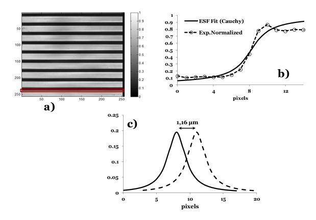
**Figure 4.6** a) Image of a diffraction grating structure; b) ESF function of a knife edge , from diffraction grating (dashed line with open circles), Cauchy fitted (black line); c) PSF plot of 2 nearest resolved points.
