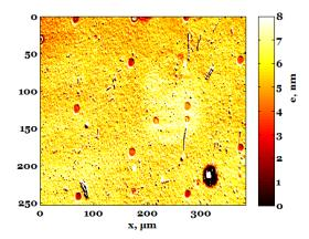
**Figure 3.14** Estimated distribution of deposited NP layer thickness resulting from the electrografting of NBD, C=0.01 M in ACN +0.1 M NBu<sub>4</sub>BF<sub>4</sub> on Au surface initially modified by 1-decanethiol (C=0.01M) and then modified by UV-lithography, for a chronoamperometric potential step between 0.3 and -0.45 V vs Ag/AgCl for 300s
