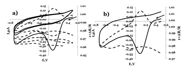
**Figure 2.6** Variation of light reflectivity during the electrografting of NBD (C=5 mM) in ACN + 0.1 M NBu4BF4 on gold microelectrode ( $\varnothing$ =250 $\mu$ m): a) black line : I=f(E), v=0.1 V/s; dashed black line: reflectivity during the electrografting; b)representation of the first cycle for CV and reflectivity (black line: I=f(E); dashed line: reflectivity variation.
