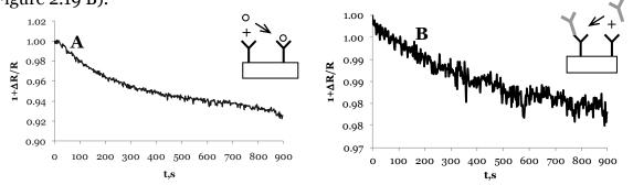
**Figure 2.19** Monitoring in real time and in situ of the interaction between the antibody of  $\alpha$ -lactalbumin (IgG) immobilized on a gold surface and  $\alpha$ -lactalbumin in solution (antigen, A) or anti IgG (B); measurements realized with 0.2  $\mu$ mol/L of a-lactalbumine (A), and with a serum of anti-IgG diluted to 1/1000 (B).
