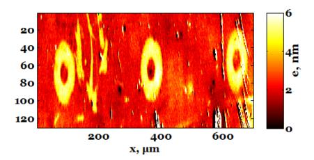
**Figure 3.12** Estimated distribution of NP layer thickness obtained from the electrografting of NBD (C=10 mM) in ACN + 0.1 M NBu<sub>4</sub>BF<sub>4</sub> on surfaces printed with BSA (C=80 $\mu$ g/mL) during a chronoamperometric potential between 0.5 and -0.4V vs Ag/AgCl for 300s.
