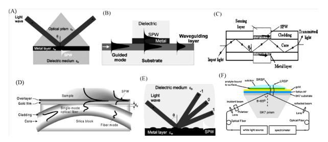
**Figure 1.2** Various SPR sensor configurations (A) Prism coupling, (B) waveguide coupling, (C) optical fiber configuration, (D) side-polished fiber coupling, (E) grating coupling, (F) long-range and short range surface plasmon (LSPR SRSP)
