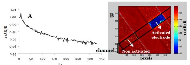
**Figure 2.20** Layer growth detection on microfluidic channel; **A:** real time monitoring of kinetics of film growth with a final thickness of about 10 nm obtained from the electrografting of a diazonium salt; **B**: reflectivity image showing the selective deposition of a thin layer (about 30 nm) on the activated gold electrode.
