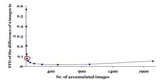
Figure 4.5 Variation of STD of difference between the 2 images in  $\Delta$  in degrees with the number of accumulated images per acquisition, for an equilibrium time of retarder, T=200ms.
