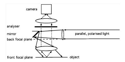
Figure 1.9 Principle of imaging ellipsometric microscopy – Neumaier's setup
