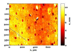
**Figure 3.15** Estimated distribution of deposited NP layer thickness resulting from the electrografting of NBD C=0.01 M in ACN +0.1 M NBu<sub>4</sub>BF<sub>4</sub> for a chronoamperometric potential step between 0.3 and -0.45 V vs Ag/AgCl for t=300s, on an Au surface previously grafted ex-situ with NBD and then locally patterned by UV-lithography.
