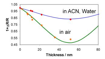
**Figure 2.5** Validation of optical model for measurements of relative reflectivity variation in air, ACN and water on Au surfaces grafted with organic layers of different thicknesses (different deposited layer thicknesses measured in air (orange rectangles) and ACN and water (red rectangles).
