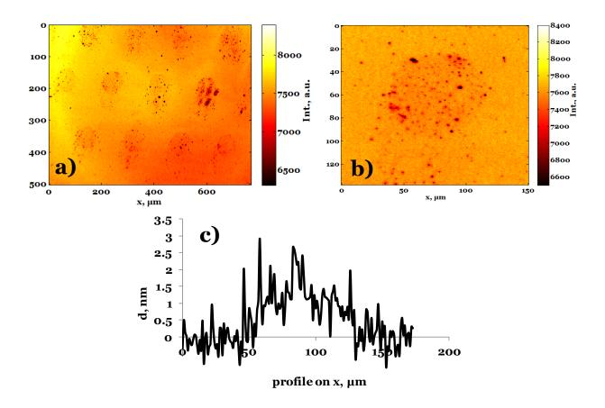
**Figure 3.3** Light reflectivity images in air of Au substrate printed with NBD (C=20 mM) in H2SO4 (1M): a) full-field image and b) magnification of a single printed spot; c) Cross-section profile (thickness) along x direction on the single spot image.
