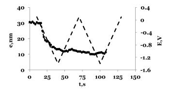
**Figure 2.16** Release of adsorbed species during the electrografting of NBD at highly negative potentials by biasing the grafted electrode in a electrolyte solution of 0.1 M NBu4BF4 in ACN between 0.1 V and -1.4 V vs Ag/AgCl.
