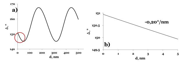
**Figure 4.4**  $\Delta$  in degrees as a function of deposited organic film thickness d on gold in liquid medium; a)  $\Delta$  variation in degrees for a deposited film of 500 nm thickness; the black line is calculated from the one layer optical model using the parameters  $\lambda$ =637 nm light, 45° incidence angle,  $n_{Au}$ =0.15+3.5i,  $n_{liq}$ =1.33,  $n_{film}$ =1.5;b) linear region of  $\Delta$  periodic variation with d (red circle in a).
