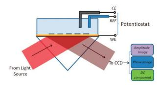
Figure 1.10 Surface impedance imaging setup
