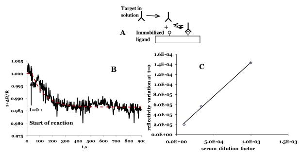
**Figure 2.18** Real time in situ evolution of the interaction between immobilized β-lactoglobuline on a gold surface with its associated antibody in a solution of rabbit serum. **A**: principle; **B**: experimental kinetic response (black) considering an adsorption kinetics. **C**: dynamic range of the immunoassay obtained from the slope (in s<sup>-1</sup>) for short intervals using Langmuir model (the starting point is at t=40 s, that corresponds to the injection of the target molecule).
