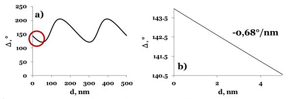
**Figure 4.3**  $\Delta$  in degrees as a function of deposited organic film thickness d on gold in air; a)  $\Delta$  variation in degree for a deposited film of 500 nm; the black line is calculated from the one layer optical model using the parameters  $\lambda$ =637 nm light, 55° incidence angle,  $n_{Au}$ =0.15+3.5i,  $n_{film}$ =1.5 b) linear region of  $\Delta$  periodic variation with d (red circle in a).
