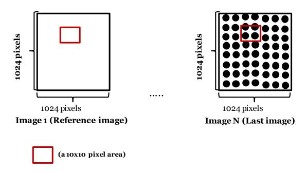
**iii)** The variation of mean intensity from pixels covering the red square is monitored for all recorded images (from Image 1 to Image N). In this way, the variation of light intensity is obtained for entire duration of the modification process applied to the surface;
