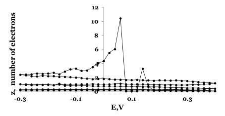
**Figure 2.9 z**, number of transferred electrons during the electrografting of the NBD (C=5 mM) in ACN + 0.1 M NBu4BF4, scan limits: 0.4 and -0.3V vs Ag/AgCl, v=0.01 V/s, on a gold microelectrode,  $\emptyset$  =25  $\mu$ m.
