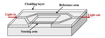
Figure 1.3 Mach-Zehnder interferometer sensor
