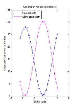
**Figure 4.2** The best fit for measured and normalized intensities (+) for imposed Nc phase shifts values (23, in our case) for the parallel (blue line) and orthogonal (red line) path used to obtain  $i^c_{\parallel}(n)$ ,  $i^c_{\perp}(n)$  from relation (1).
