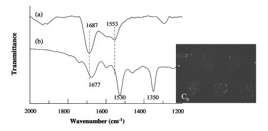
**Figure 3.19** IR spectra of adsorbed lyso on Au surface before (a) and after (b) deposition of the blocking layer; C<sub>b</sub>—the fluorescence response of lyso Au surface incubated with a fluorescent labeled anti-lyso aptamer.
