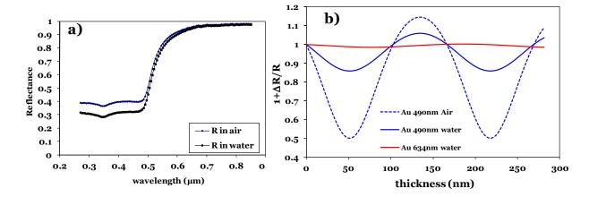
**Figure 2.3** a) Reflectivity spectrum of a bare gold surface in air and water; b) Theoretical relative variations of reflectivity as function of deposited layer thickness on gold surface and wavelength of light beam (blue or red spectral regions) and optical indexes of the media where the light is propagated (air and water).
