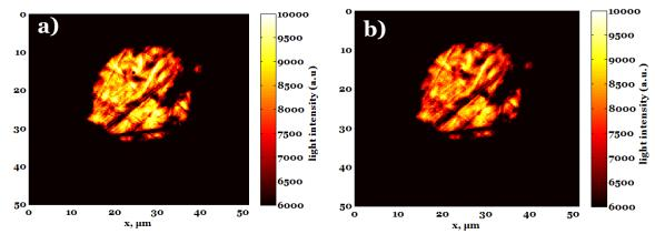
**Figure 2.7** Light intensity image of a gold microelectrode ( $\varnothing$ =25 µm) a) before grafting; b) after grafting of NBD, (C=5 mM) in ACN + 0.1 M NBu4BF4, chronoamperometry (CA) potential step from 0.2V to -0.3 V vs Ag/AgCl, for a duration of 300s.
