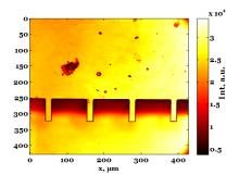
Figure 3.9 Light Reflectivity intensity image in air of a cantilever platform
