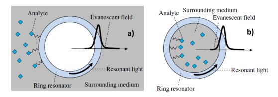
**Figure 1.5** The principle of optical ring resonator sensor: the light circulating along the resonator and its evanescent field is present in the surrounding medium outside (a) or inside (b) the ring resonator, interacting with the analyte on the ring resonator exterior surface (a) or interior surface (b) and in the surrounding medium
