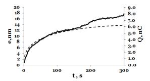
**Figure 2.9** Evolution of the thickness (plain line) and charge (dashed line) for the deposition of a nitrophenyl film (NP) during a chronoamperometric potential step between 0.3 and -0.3 V vs Ag/AgCl for 300s at a gold microelectrode ( $\varnothing$ =25 µm) of NBD (C=5 mM) in ACN + 0.1 M NBu4BF4.
