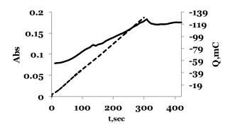
**Figure 2.13** Electrografting of NBD (C=5 mM) in ACN + 0.1 M NBu4BF4 on an ITO electrode, for a chronoaperometric potential step between 0.5 and -1.2V vs Ag/AgCl, t=300s; black line: absorption; dashed line: charge consumed.
