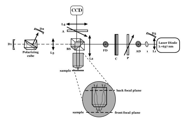
**Figure 4.1** Setup of the ellipsometric microscope: AD-aperture diaphragm (iris diaphragm); P-polarizer at 45°; C – used as Babinet-Soleil compensator or liquid crystals variable retarder (Meadowlark); FD-field diaphragm; 1- spinning ground glass diffuser; BS – beam splitter; D1, D2,D3 – photodiodes; A – analyzer; L1-L4 – lenses.
