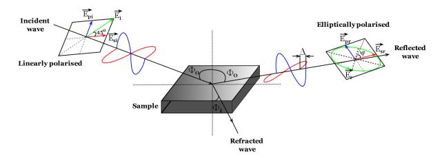
**Figure 1.8** Ellipsometry principle: p, s-parallel and perpendicular direction of light components to the plan of incidence;  $\Phi_0$ -incidence angle;  $\Phi_1$  – refractive angle
