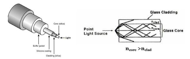
Figure 1.6 The schematic of an optical fiber
