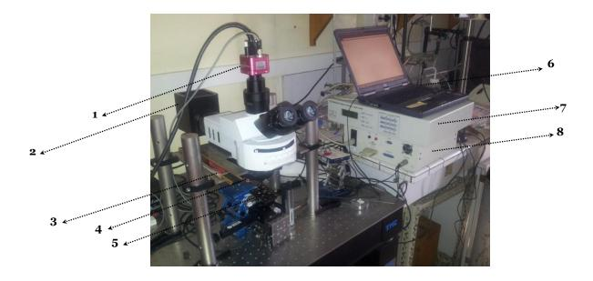
The proposed configuration for the light reflectivity measurements
