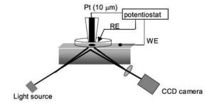
**Figure 1.14** Schematic diagram of SECM and SPR-i configuration : RE-reference electrode, WE-working electrode
