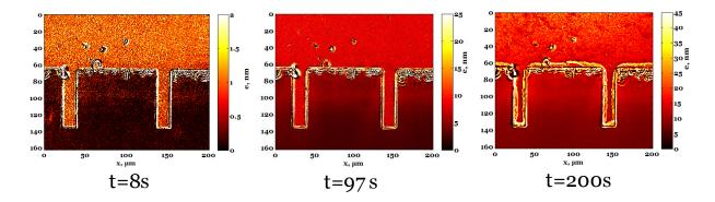
**Figure 3.10** Layer thickness images estimated from light reflectivity images recorded during the electrografting of NBD, C=5 mM in ACN + 0.1 M  $NBu_4BF_4$  for a chronoamperometric potential step between 0.3 and -0.7 V vs Ag/AgCl .
