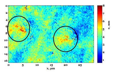
**Figure 4.14** The thickness in nm of the deposited organic layer at the end of diazonium electro-grafting (difference between last and first image)
