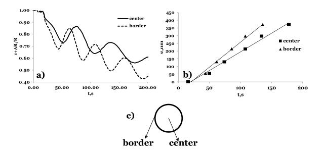
**Figure 3.8** Variation with time of NP layer film growth at (c) different regions of a microdisk electrode ( $\emptyset$ =250µm) during NP film growth by electrografting of NBD salt (C=5 mM) in ACN + 0.1 M NBu<sub>4</sub>BF<sub>4</sub> for a chronoamperometric potential step between 0.5 and -1.1V vs Ag/AgCl. a) experimentally accessed local light reflectivity change, b) time evolution of the NP layer thickness estimated at the maxima and minima of a).
