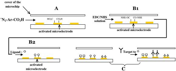
**Figure 2.21** Example of an immunoassay in a microfluidic cell: preparation of a platform with multi-ligands by repetition of the procedures from step A+B: A: selective electrografting of an initial attaching layer by electrochemical selective activation of a microelectrode; B1+B2: Selective coupling of a ligand; C: Multiple detection of a biological target present in a mixture solution.
