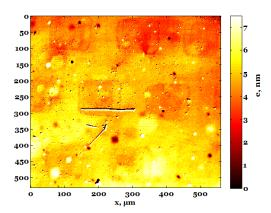
**Figure 3.11** Estimated image of the distribution of the thickness of a NP layer grown from the electrografting of NBD (C=0.01 M) in H2SO4 (C=0.01M) on a  $\mu$ CP printed Au surface with 1-decanethiol (C=0.01 M) by 100x100  $\mu$ m² stamps spaced by 100  $\mu$ m, for a chronoamperometric potential step between 0.5 and -0.4 V for 300s.
