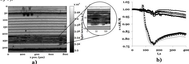
**Figure 2.11** Electrografting of NBD (C=5 mM) in ACN + 0.1 M NBu4BF4 on gold microarray electrodes for a chronoamperometric potential step between 0.3 V and -0.9 V vs Ag/AgCl for 400s.
