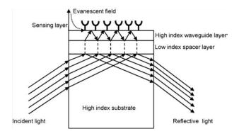
Figure 1.4 Resonant mirror structure
