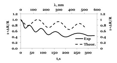
**Figure 2.15** Comparison of experimental (black line) showed in Fig.2.11, and theoretical (dashed line) light reflectivity for  $\lambda$ =490 nm with a deposited film thickness (only for theoretical variation).
