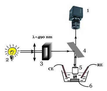
**Figure 2.4** Schematic representation of the setup used for measuring relative variations of light reflectivity.
