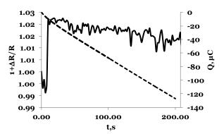
**Figure 2.10** Electrografting of DMBD, C=5 mM in ACN+ 0.1M NBu4BF4, to an Au microelectrode ( $\varnothing$ =250 µm), chronoamperometric potential step between 0.5 and -0.7V vs Ag/AgCl, t=200s; plain line - variation of light reflectivity during the electrografting; dashed line: the consumed charge during the electrografting reaction
