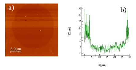
**Figure 3.16** a)AFM image of a single pattern ( $\emptyset$  = 24  $\mu$ m); b) diameter profile of the analyzed spot;
