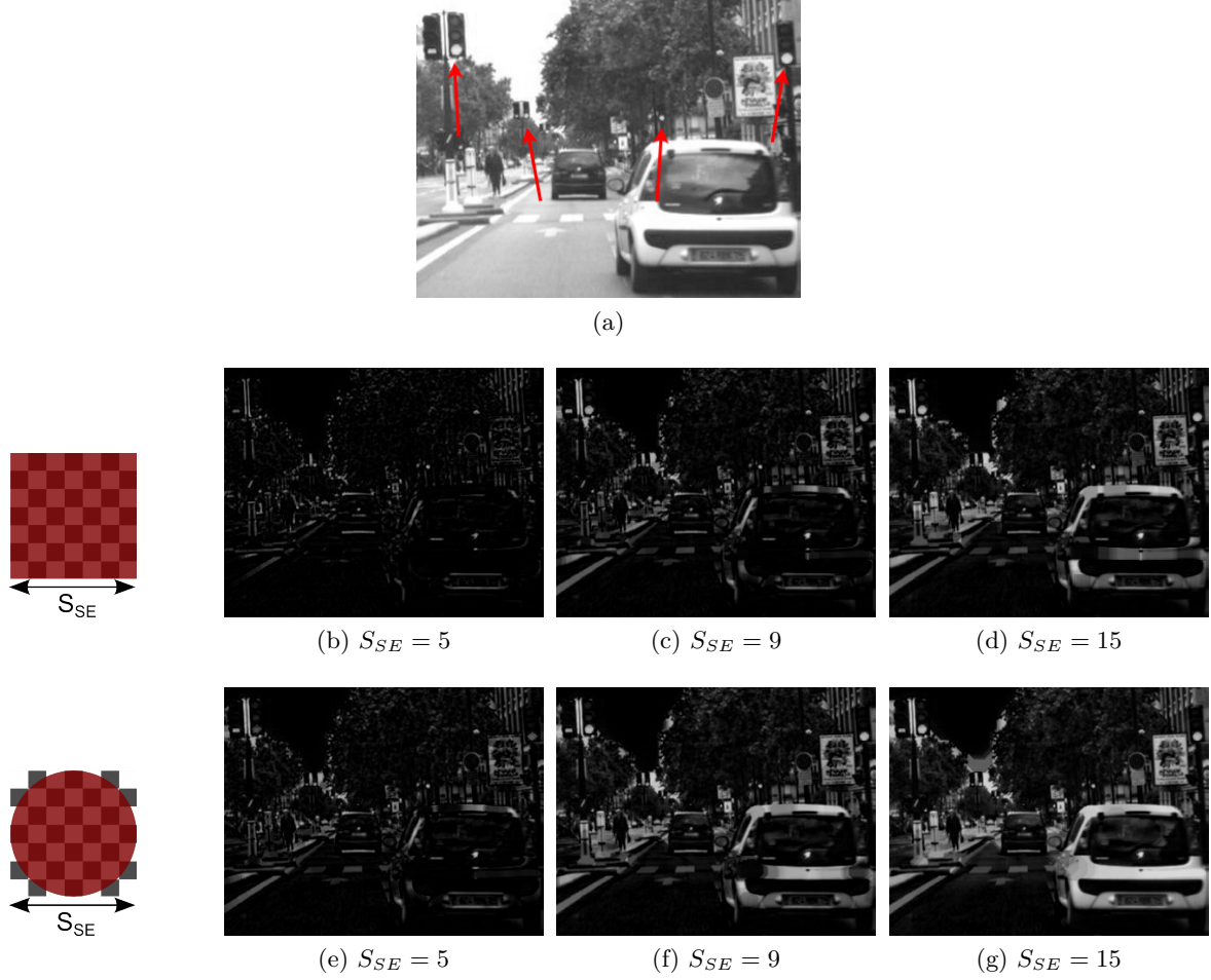
Figure 4.11: Cropped picture of a typical urban scene with traffic lights at different distance from the camera. (a) is the sample picture and (b)-(g) are samples white top hat output with structuring elements of varying size. Note that when S_{SE} = 5 the large spots (i.e. corresponding to close traffic light) are not segmented (b) and (e). Additionally one may see that the top hat is different with a square (b-d) or a circular element (e-g) though the spots are segmented identically.
