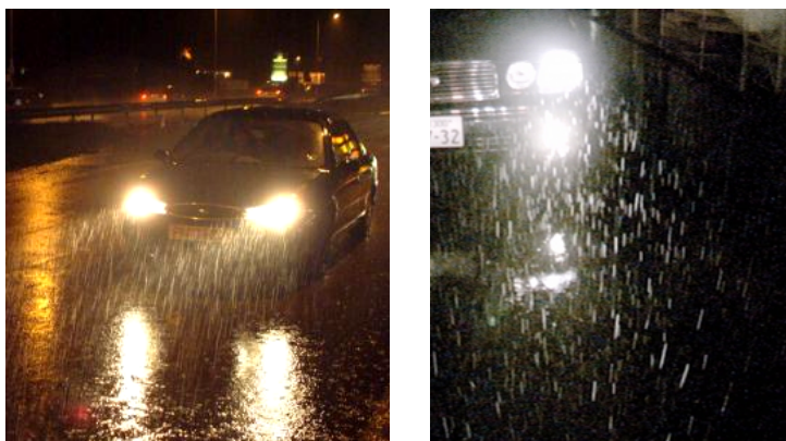
Figure 3.1: At night, illuminated rain appears as a bright flickering (distracting) pattern that reduces driver visibility.
