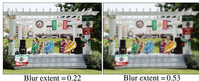
Figure 2.6: Difference of gradients to detect defocus blur using [Crete et al., 2007]. Left is a sharp version of a picture. Right is an digitally blurred version. The method correctly ranks the right picture as blurrier using the difference of derivatives.
