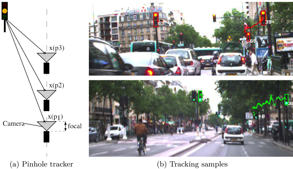
Figure 4.29: Tracking using pinhole approximation. (a) scheme of the pinhole tracker. (b) example of traffic lights tracked. The dots indicate the previous positions of the traffic lights. Note, that if no pitch occurred the history points should be perfectly linear.
