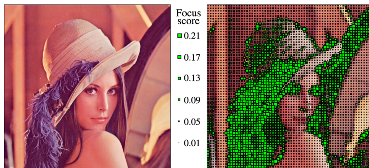
Figure 2.8: Spectral analysis to detect defocus blur using weighted frequencies in patches of 8 \times 8 to highlight the element in focus. Note that even sharp regions have focus values close to 0. Source: [Dai and Wu, 2007].
