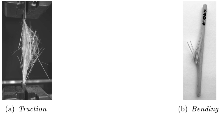
FIG. 3.2.1 – Glass fibers reinforced vinylester samples' static rupture modes in traction and bending.
